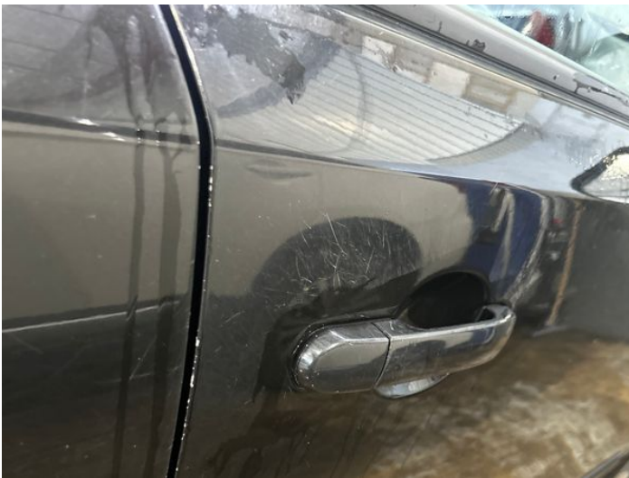
5: Door osf Chipped Edge Chip
