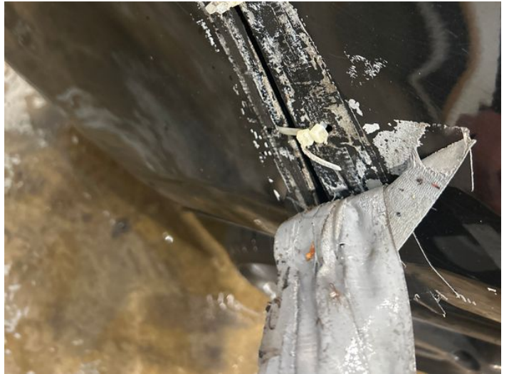
16: Wing nsf Hole UpTo 10mm
