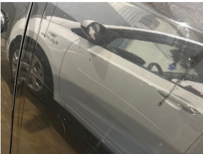
13: Door nsr Scratched Over 25mm Thru Paint
