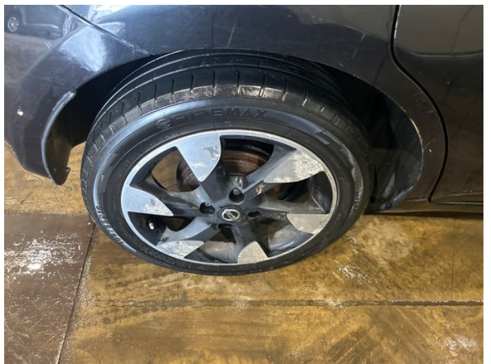
8: Wheel osr Corroded Light
