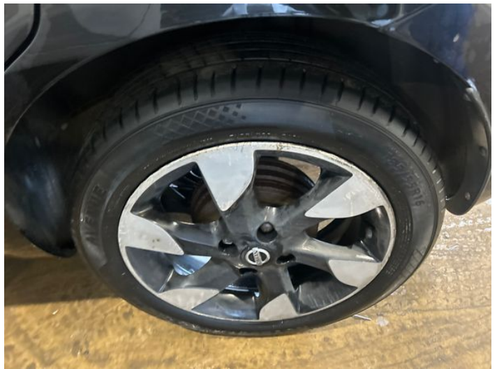
12: Wheel nsr Corroded Light
