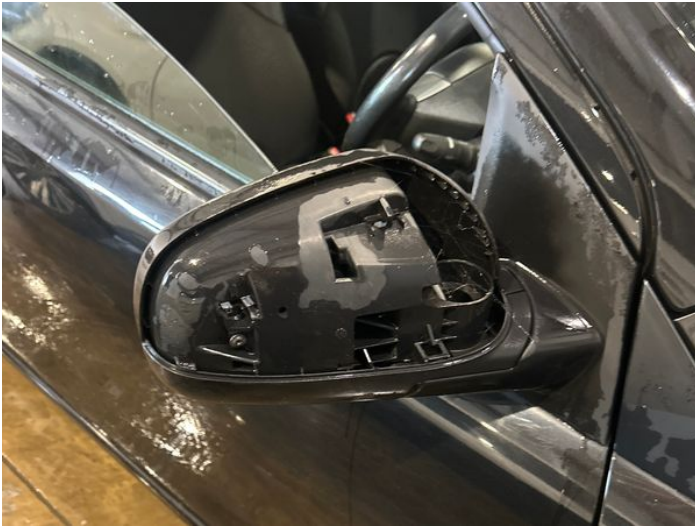
3: Door Mirror Assy osf Missing Replace
