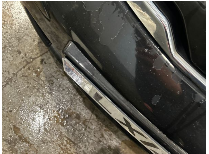
18: Bumper Front Poor Previous Repair Paint Flake
