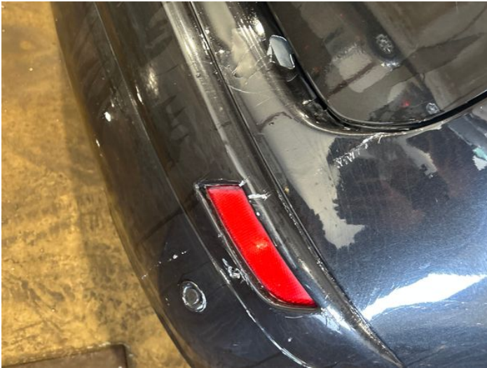
9: Bumper Rear Poor Previous Repair Paint Flake
