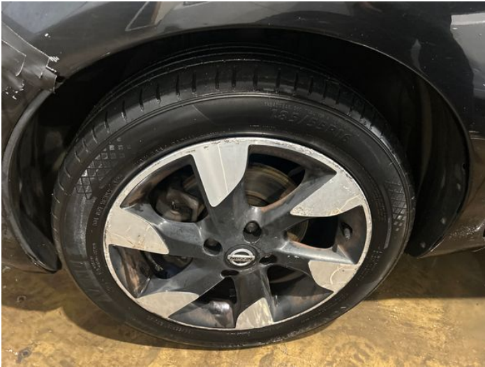
15: Wheel nsf Corroded Light
