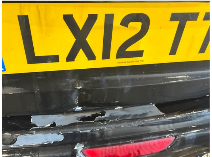
10: Tailgate Dented With Paint Damage
