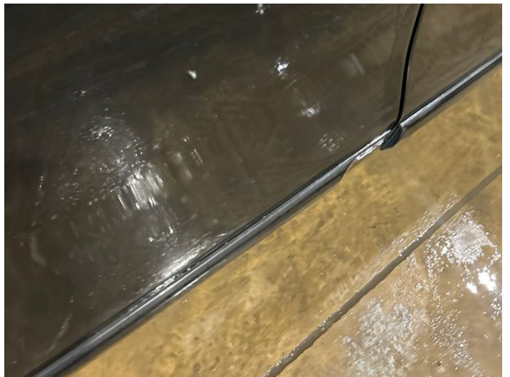
6: Door osr Chipped Multiple Chips
