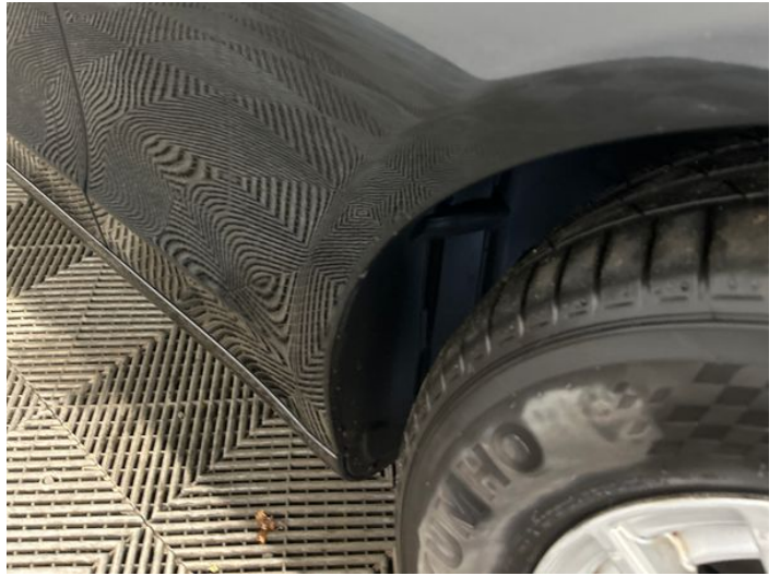
4: Wing osf Poor Previous Repair Poor Paint
