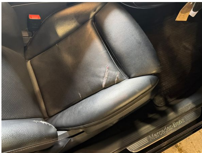
1: Seat Base Cover osf Torn Over 3mm
