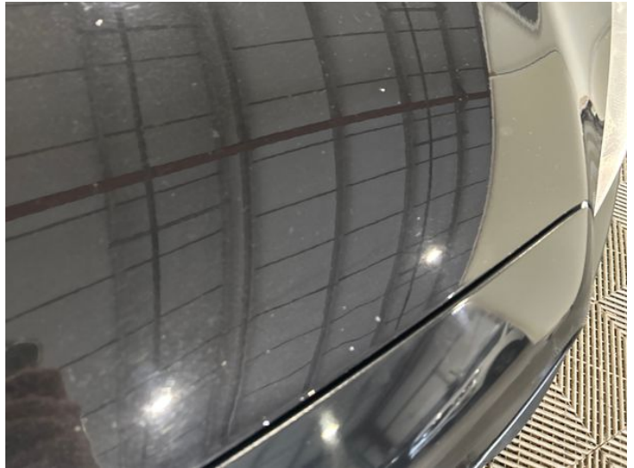
16: Bonnet Chipped Multiple Chips
