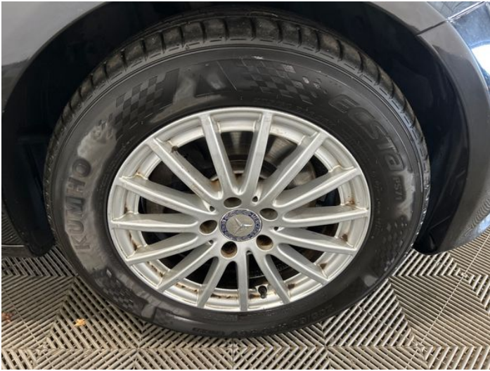
3: Wheel osf Scratched Over 50mm
