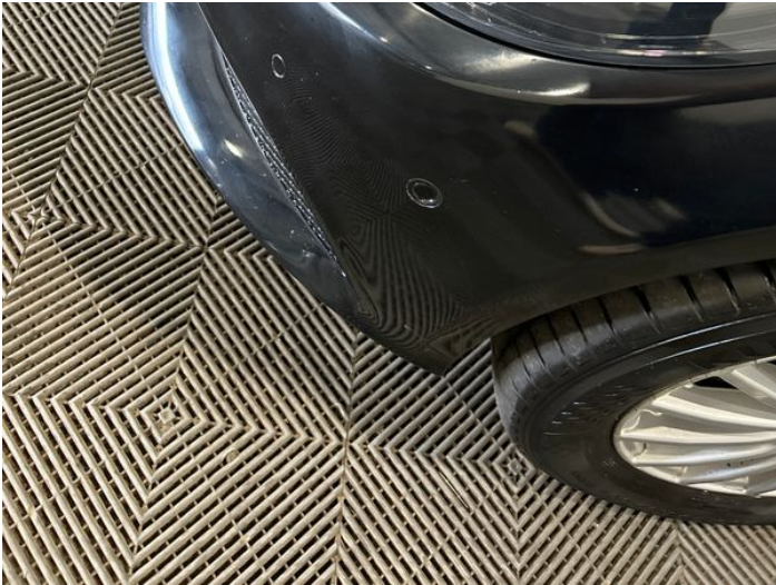
15: Bumper Front Poor Previous Repair Poor Paint
