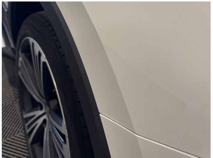
12: Qtr Panel nsr Dented 2 Or Less UpTo 10mm
