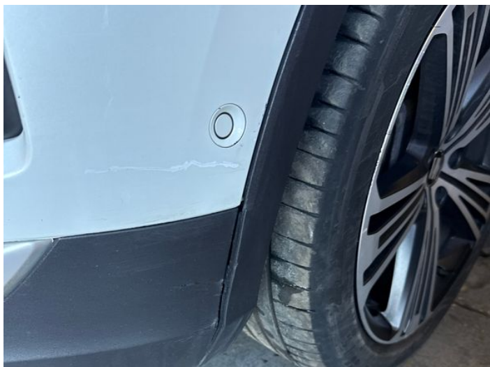
21: Wing Front Arch Extension ns Scuffed (Unpainted) Over 100mm
