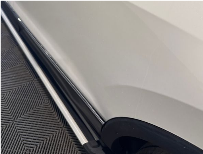
9: Door nsr Poor Previous Repair Poor Paint
