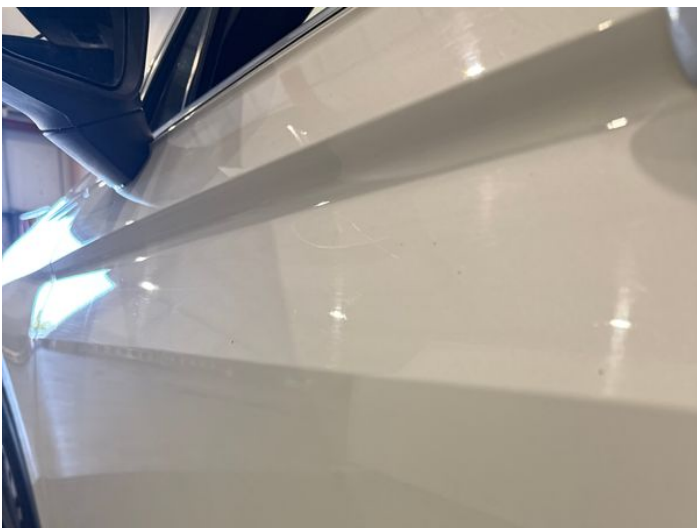
7: Door nsf Dented Between 10mm + 30mm
