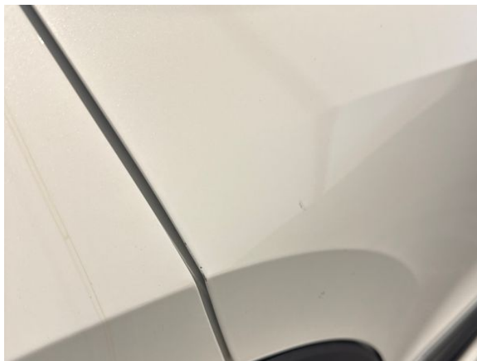
16: Door osr Chipped Edge Chip
