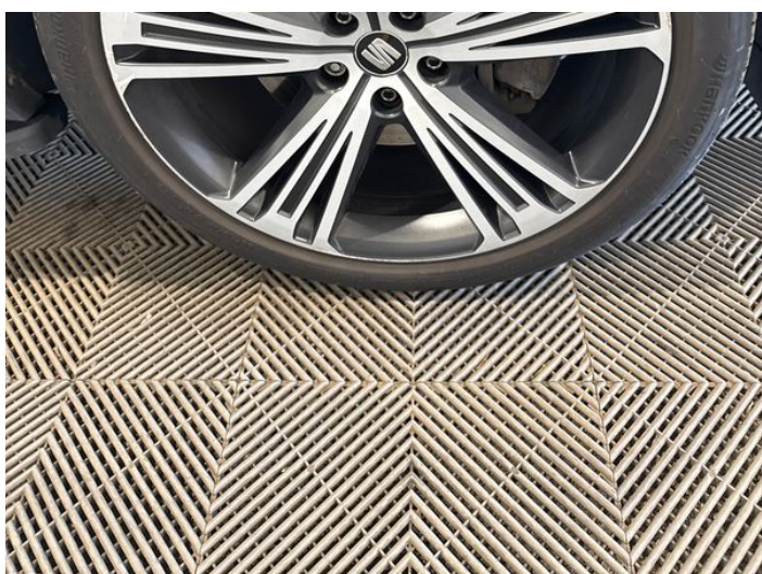
19: Wheel osf Scratched Over 50mm
