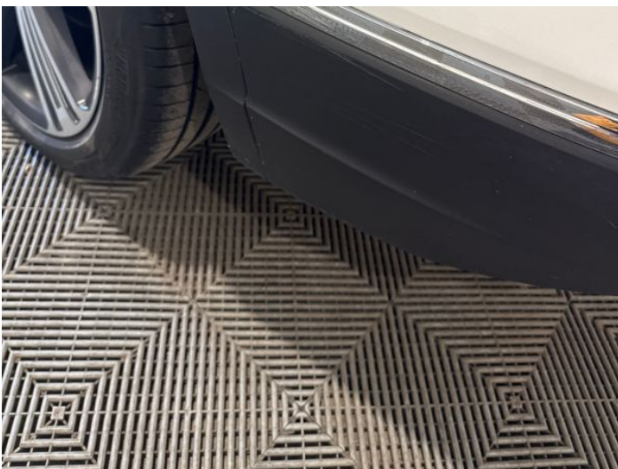
13: Bumper Rear Moulding Scuffed (Unpainted) Over 100mm
