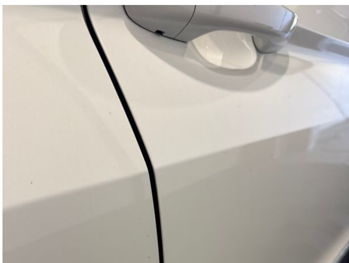
17: Door osf Chipped Edge Chip
