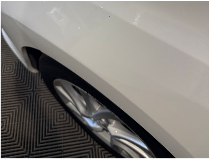
5: Wing nsf Chipped 1 To 5
