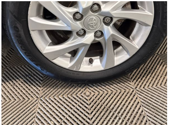
10: Wheel nsr Scratched Over 50mm
