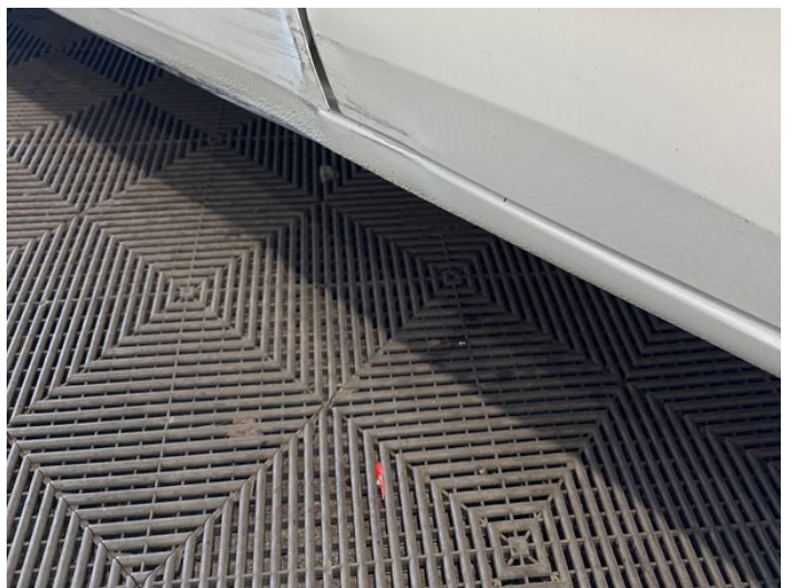
8: Door nsr Dented With Paint Damage
