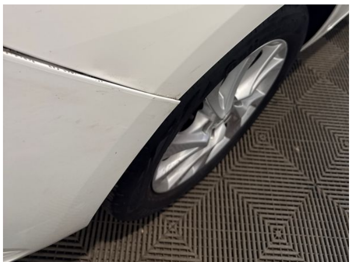
14: Qtr Panel osr Dented Between 10mm + 30mm
