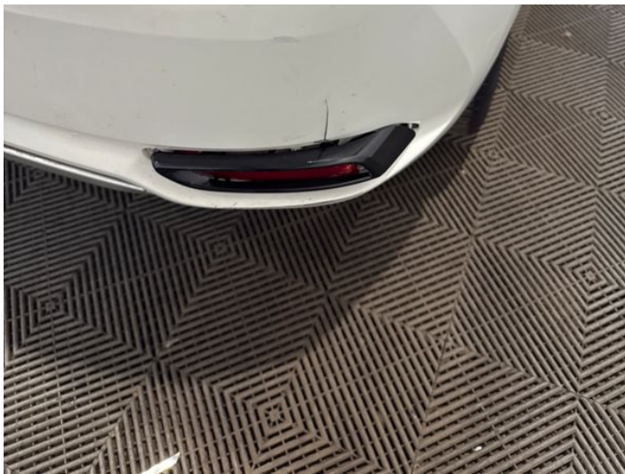
11: Bumper Rear Cracked Over 25mm
