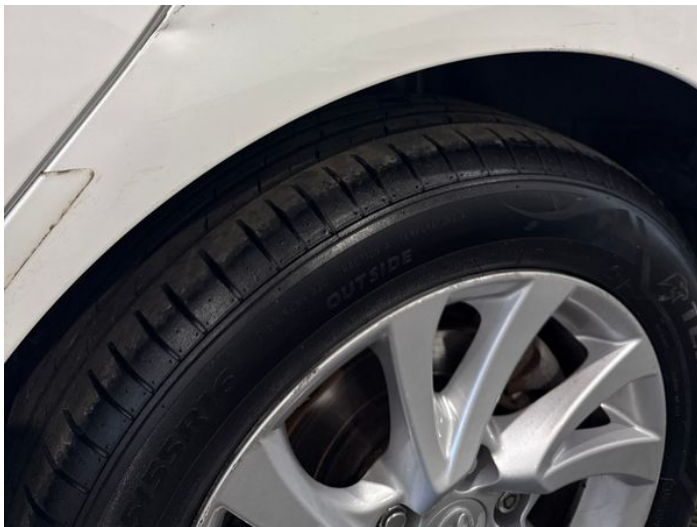
9: Qtr Panel nsr Dented With Paint Damage
