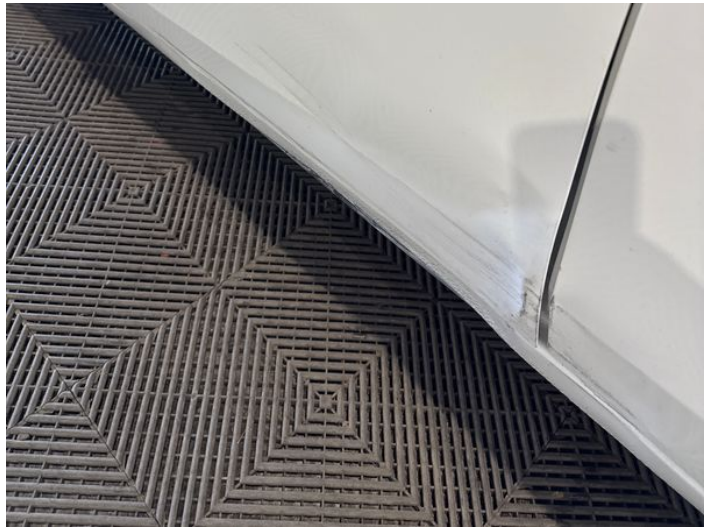
6: Door nsf Dented With Paint Damage
