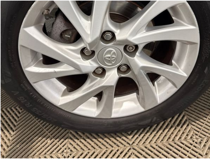
15: Wheel osr Scratched Over 50mm
