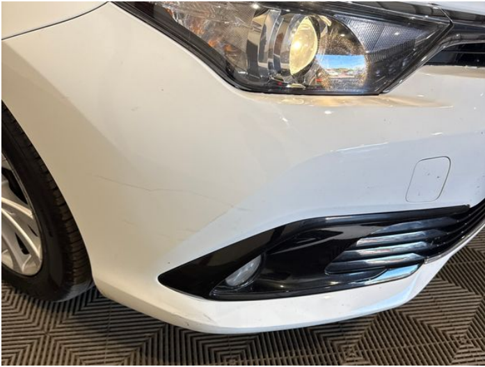
3: Bumper Front Scratched Over 100mm Thru Paint
