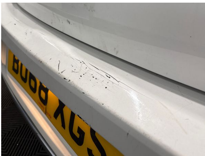
13: Tailgate Scratched Over 25mm Thru Paint
