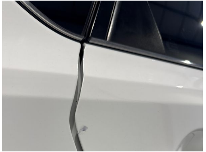
16: Door osr Scratched UpTo 25mm Thru Paint
