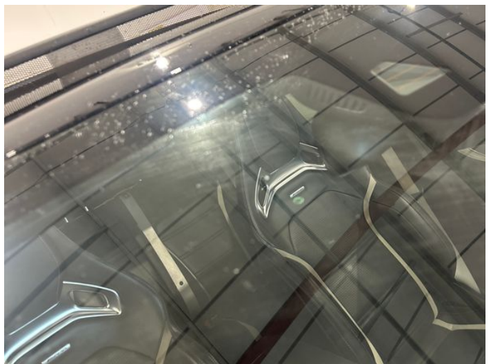
8: Screen Front Chipped UpTo 10mm
