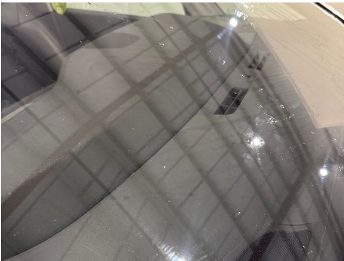
17: Screen Front Chipped UpTo 10mm
