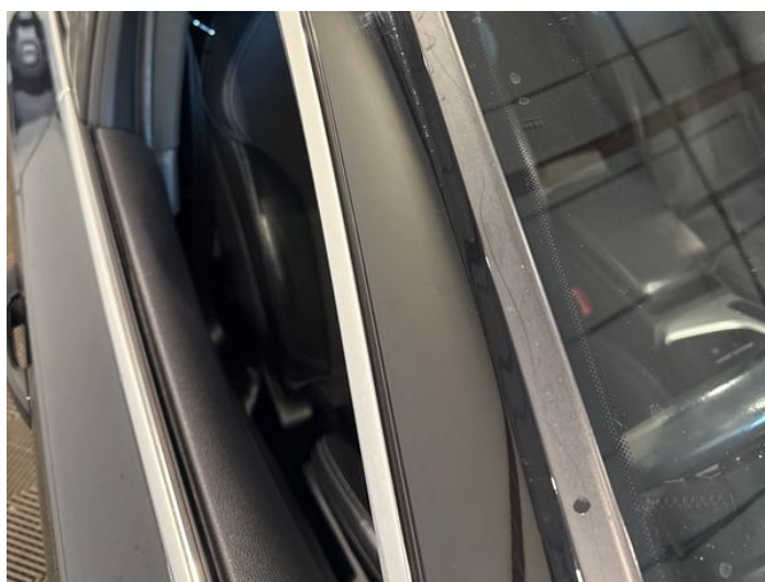
18: A Post os Scratched Over 25mm Thru Paint
