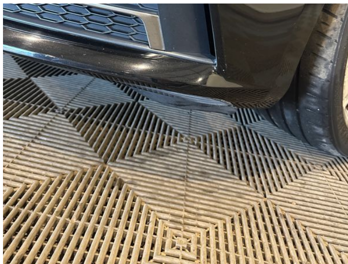
2: Bumper Front Scratched 25 to 100mm Thru Paint
