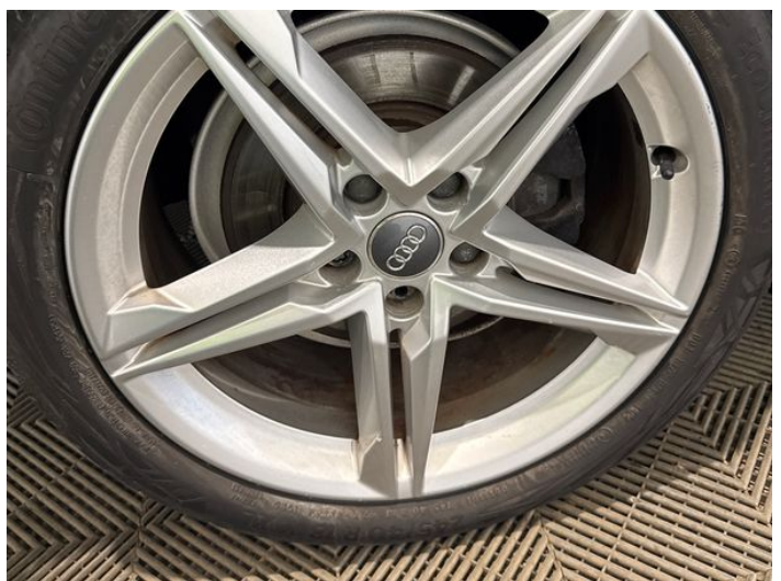
14: Wheel osr Scratched Over 50mm
