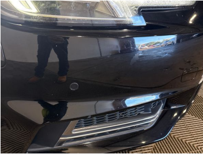
3: Bumper Front Scratched 25 to 100mm Thru Paint
