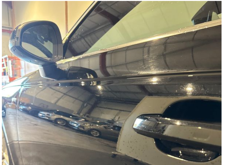
6: Door nsf Dented Between 10mm + 30mm
