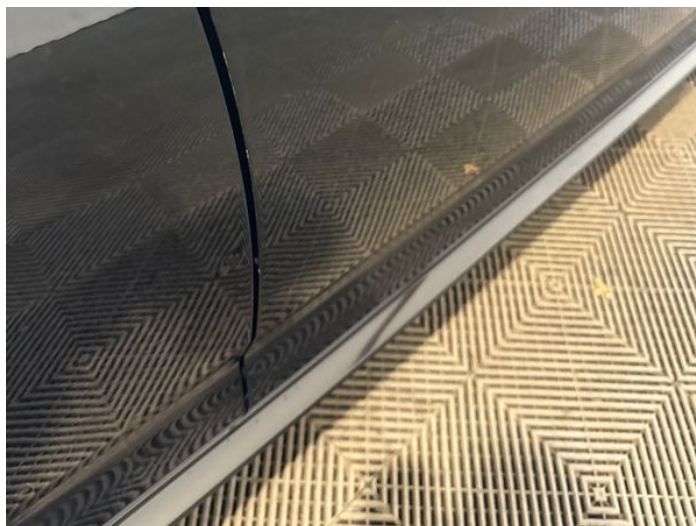
16: Door osf Chipped Edge Chip
