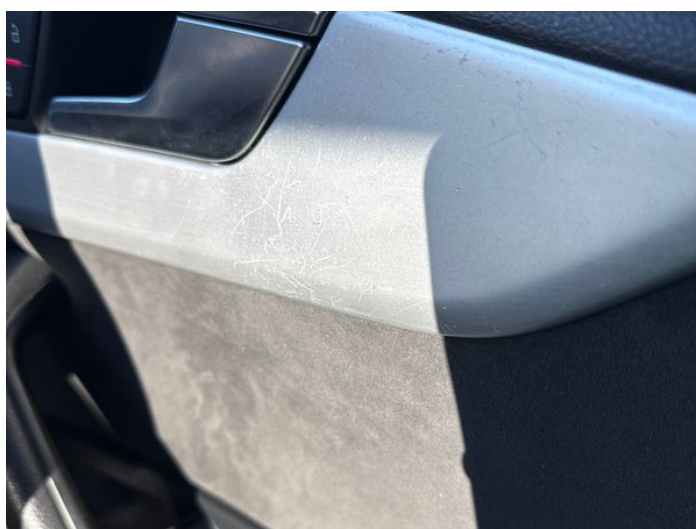
20: Door Pad osf Scuffed Over 25mm
