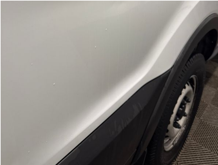
15: Qtr Panel osr Dented Over 30mm
