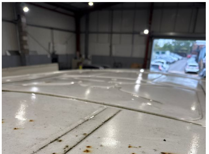
14: Roof Dented With Paint Damage
