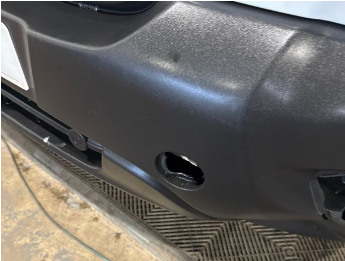
3: Front TowEye Cvr Missing Replace
