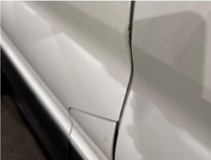
9: Door nsf Chipped Edge Chip
