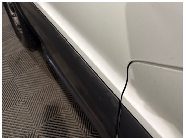
8: Door nsf Dented Between 10mm + 30mm
