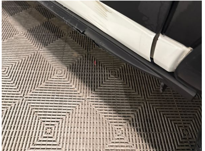
10: Door nsr Dented With Paint Damage
