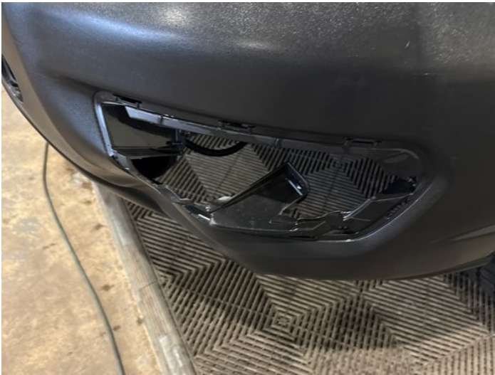
5: Fog Lamp Surround ns Missing Replace
