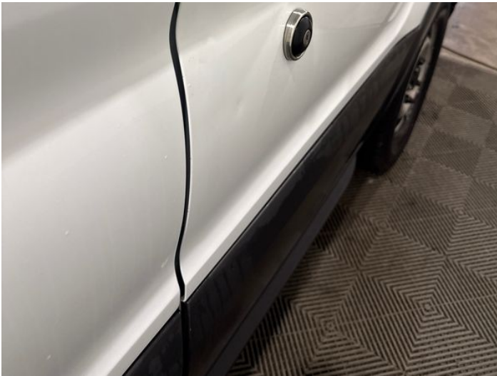
17: Door osf Dented With Paint Damage
