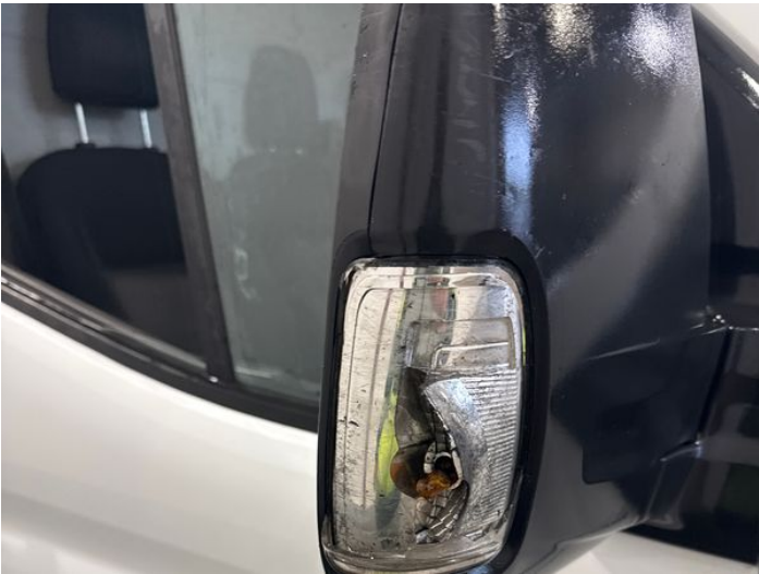
18: Flasher Side Repeater os Broken Replace
