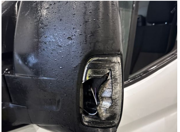
6: Flasher Side Repeater ns Broken Replace
