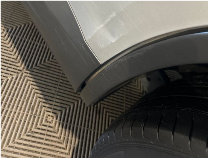
9: Door nsr Dented With Paint Damage
