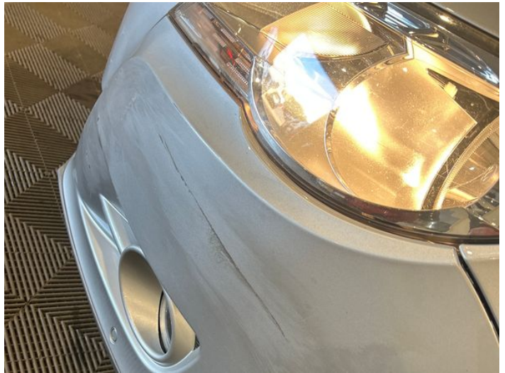
12: Bumper Front Poor Previous Repair Poor Paint
