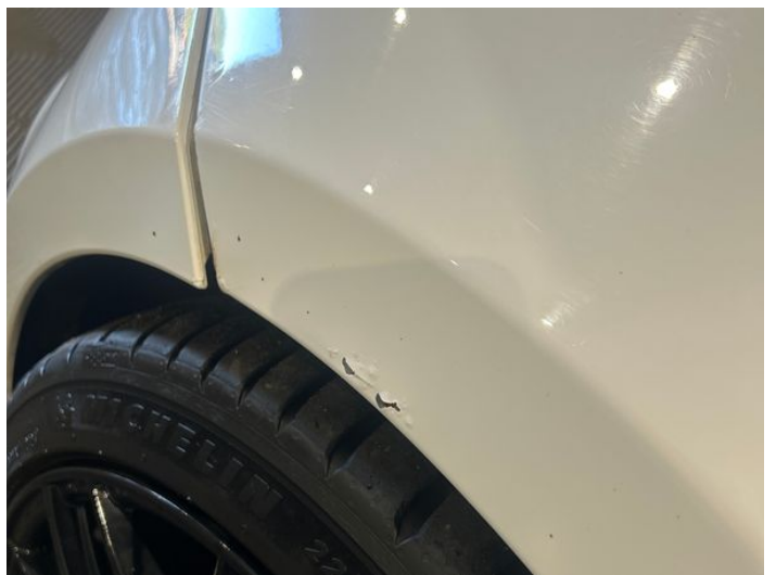
8: Wing nsf Poor Previous Repair Paint Flake
