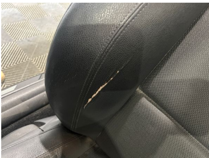
13: Seat Back Cover osf Scuffed Over 25mm
