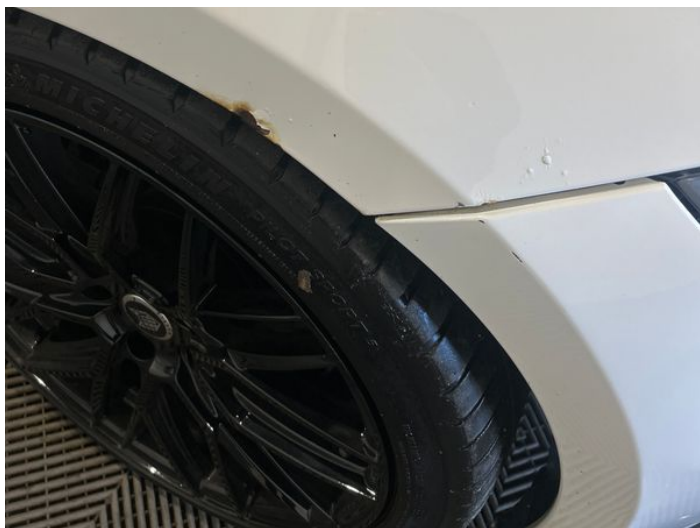
1: Wing osf Rusted Over 5mm
