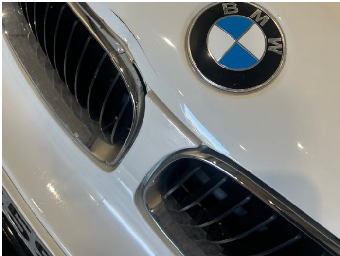
9: Bonnet Dented With Paint Damage
