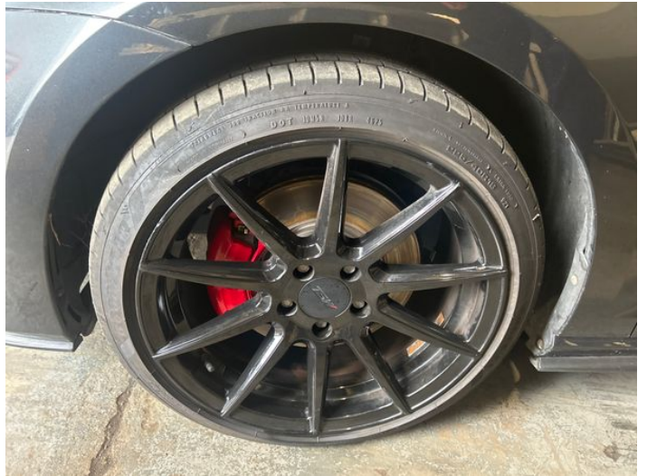
10: Wheel nsf Scratched Over 50mm
