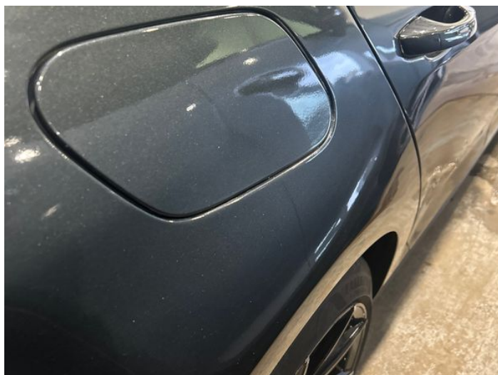
6: Qtr Panel osr Poor Previous Repair Poor Paint
