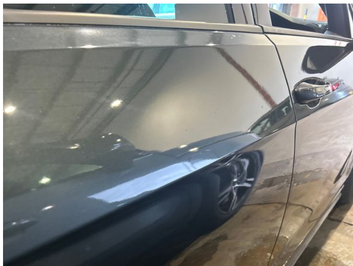
4: Door osr Poor Previous Repair Poor Paint
