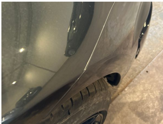
2: Wing osf Poor Previous Repair Poor Paint
