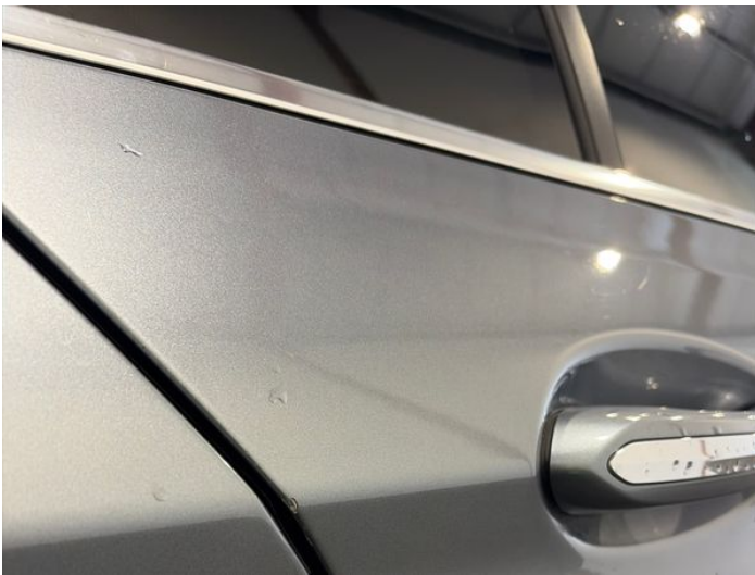
11: Door osr Chipped Edge Chip
