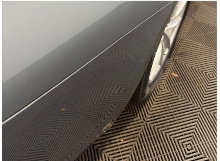
10: Qtr Panel osr Dented Over 2 UpTo 10mm
