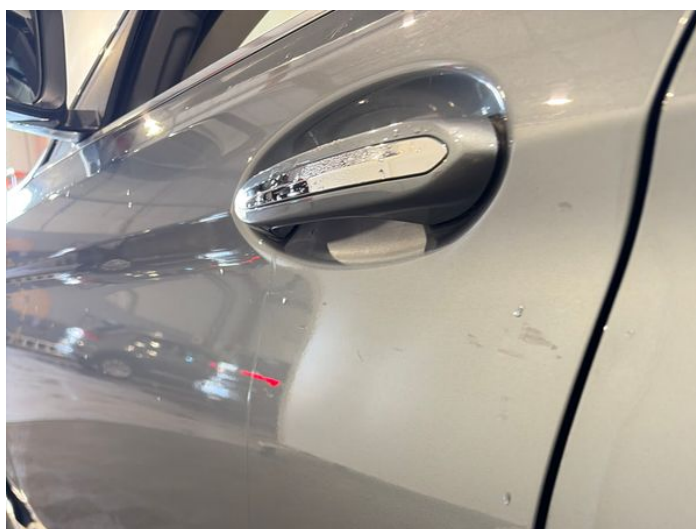
6: Door nsf Dented With Paint Damage
