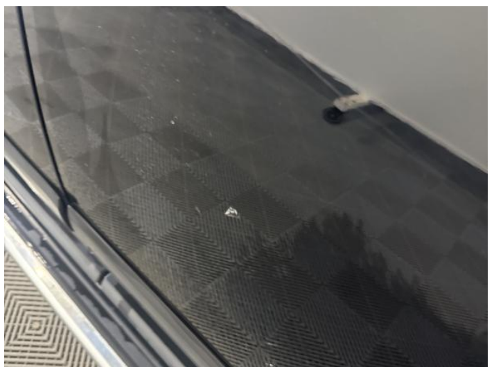
8: Door nsr Scratched UpTo 25mm Thru Paint
