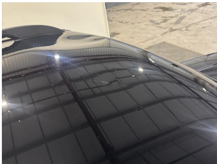
16: Roof Dented Between 10mm + 30mm
