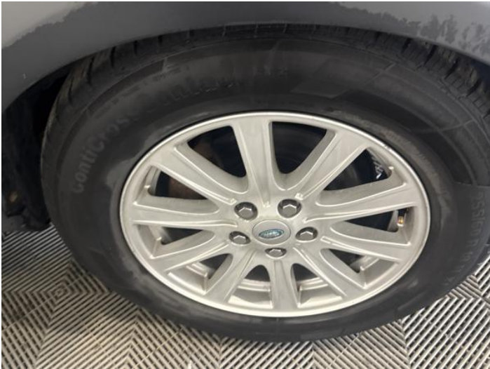
21: Wheel osf Scratched Over 50mm
