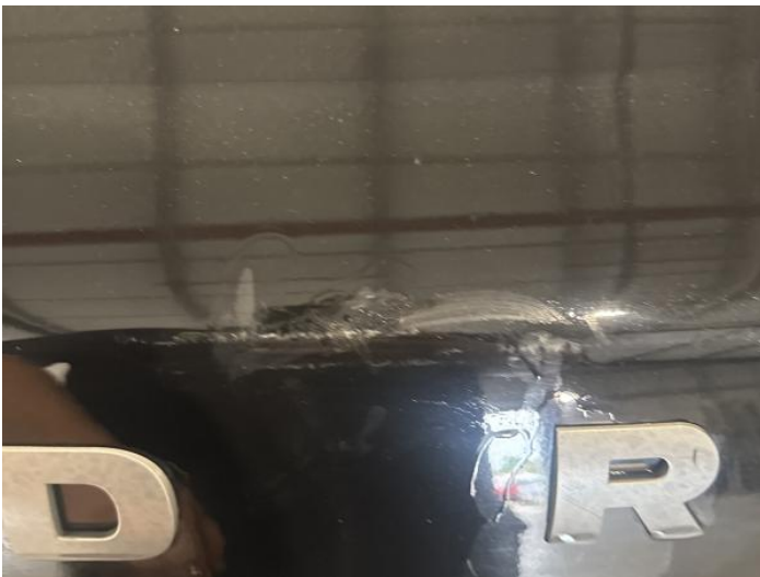
1: Bonnet Scratched Over 25mm Thru Paint
