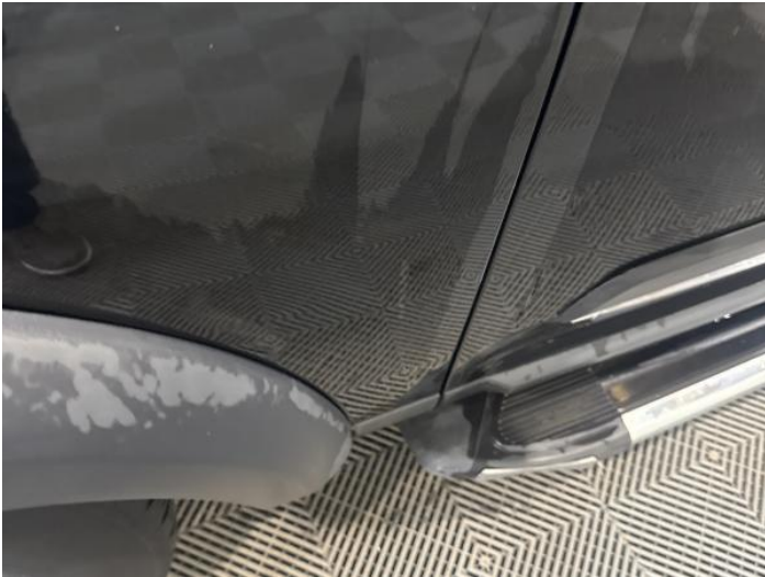
3: Wing nsf Dented Between 10mm + 30mm
