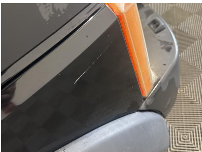
19: Wing osf Scratched Over 25mm Thru Paint
