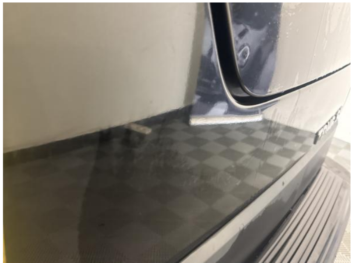
12: Boot Lid Dented 2 Or Less UpTo 10mm
