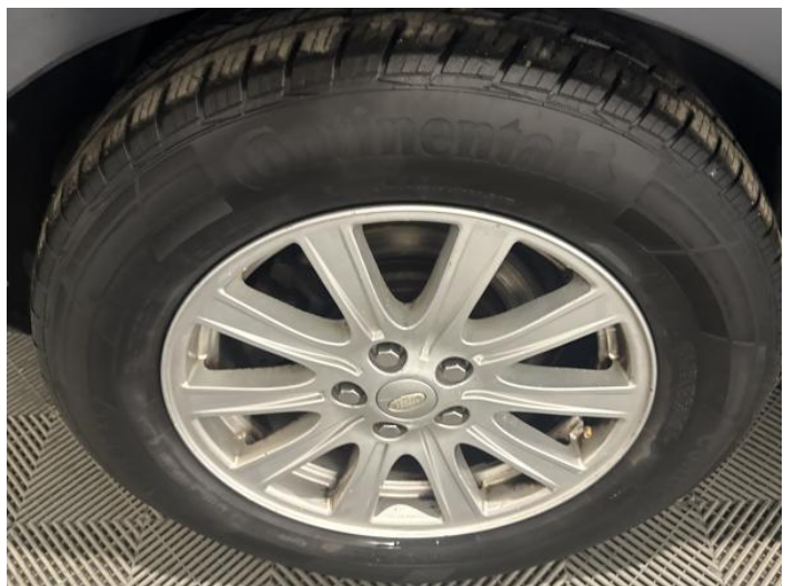
14: Wheel osr Scratched Over 50mm
