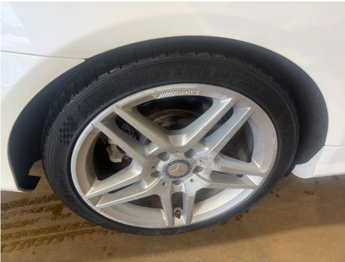
5: Wheel osr Scratched Over 50mm
