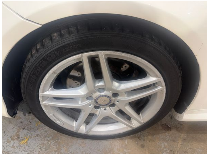
10: Wheel nsf Scratched Over 50mm
