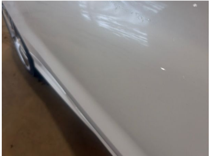
4: Door osf Dented Over 2 UpTo 10mm
