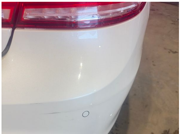
14: Bumper Rear Scratched 25 to 100mm Thru Paint
