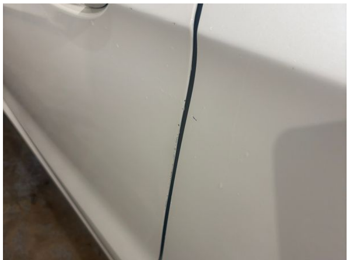
8: Door nsf Chipped Edge Chip
