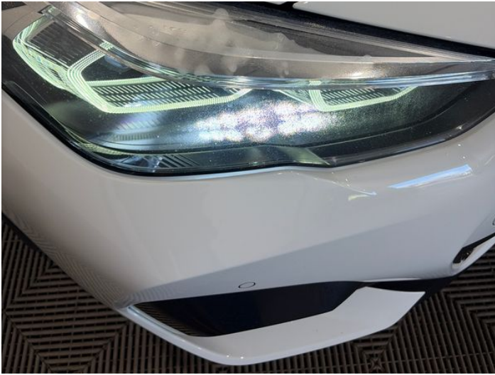
3: Other N/A N/A Condensation in headlight
