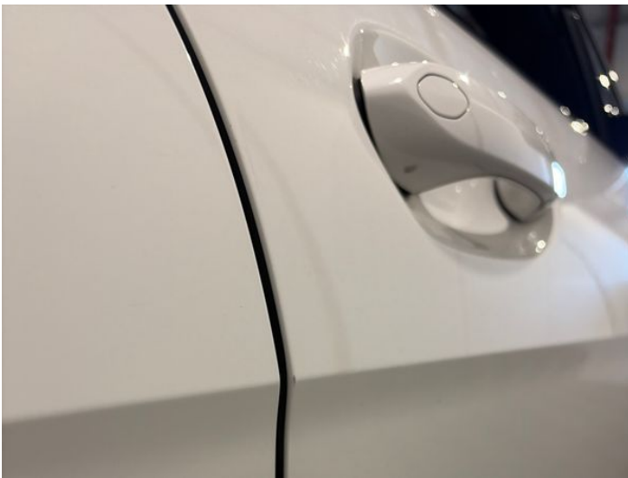
11: Door osf Chipped Edge Chip
