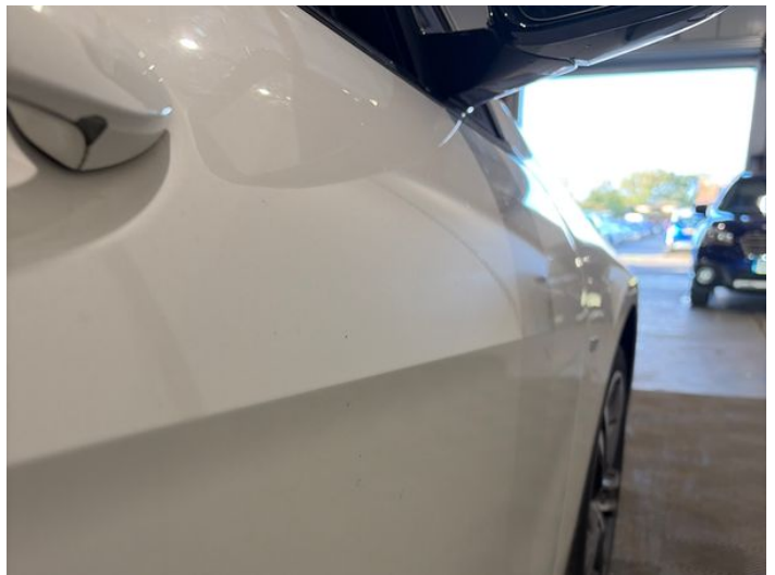
12: Door osf Dented Over 2 UpTo 10mm
