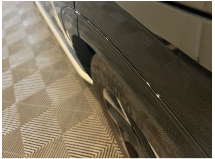
6: Qtr Panel nsr Dented Between 10mm + 30mm
