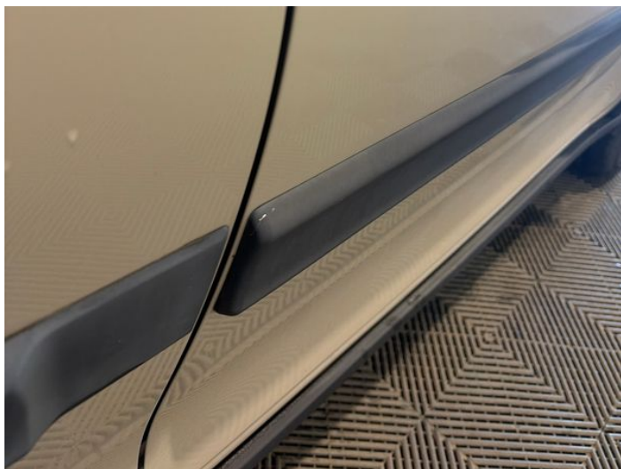
1: Door osf Chipped Edge Chip
