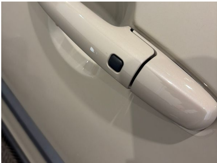
3: Handle Outer nsf Scratched (Painted) UpTo 25mm Thru Paint
