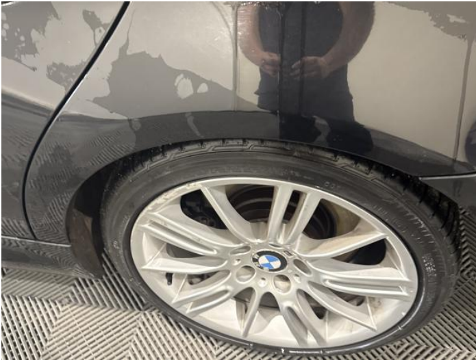
9: Wheel nsr Scratched Over 50mm
