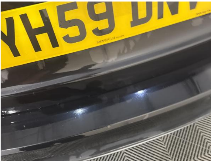
11: Bumper Rear Scratched 25 to 100mm Thru Paint
