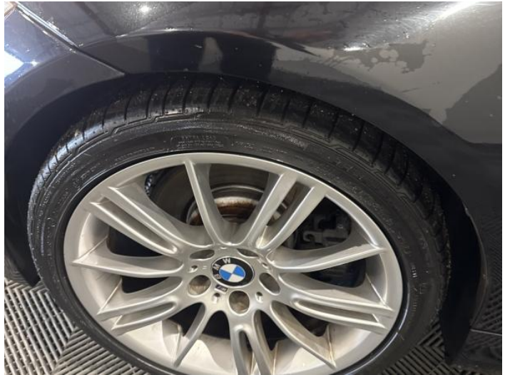
4: Wheel nsf Scratched Up To 50mm
