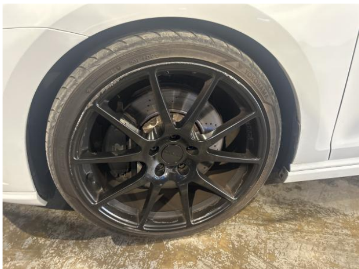
9: Wheel nsf Scratched Over 50mm
