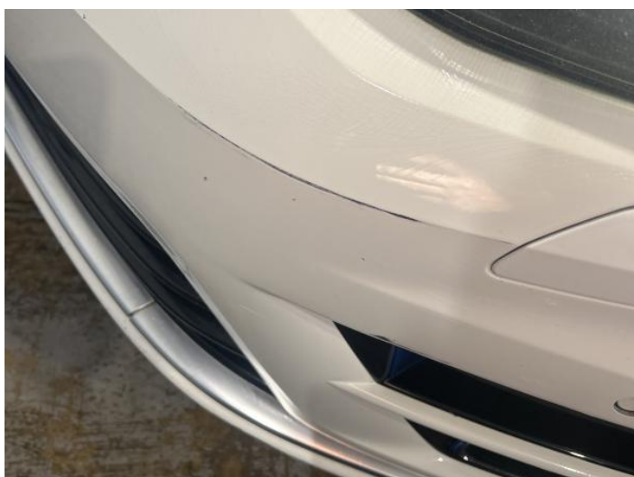
11: Bumper Front Scratched 25 to 100mm Thru Paint
