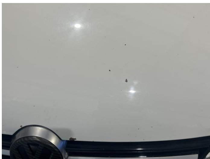
12: Bonnet Chipped Multiple Chips
