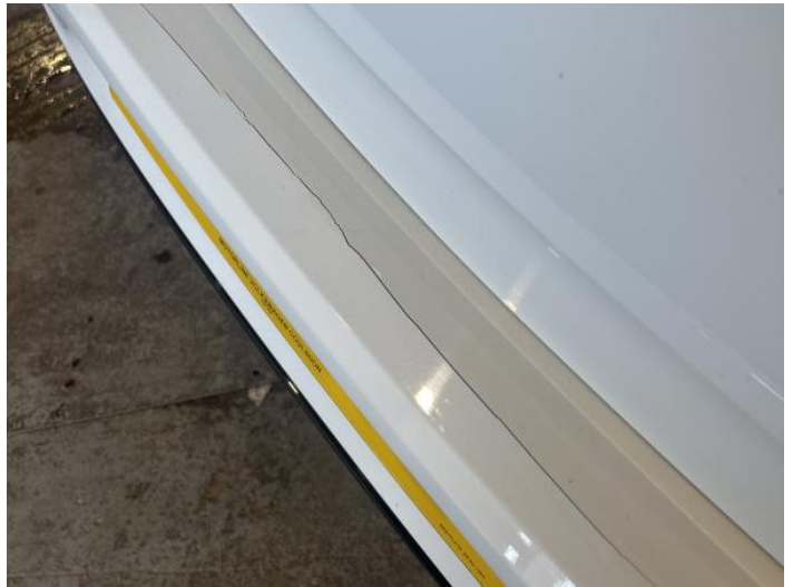
6: Bumper Rear Poor Previous Repair Paint Flake
