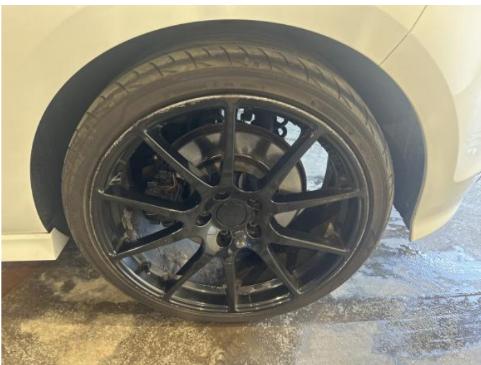
7: Wheel nsr Scratched Over 50mm
