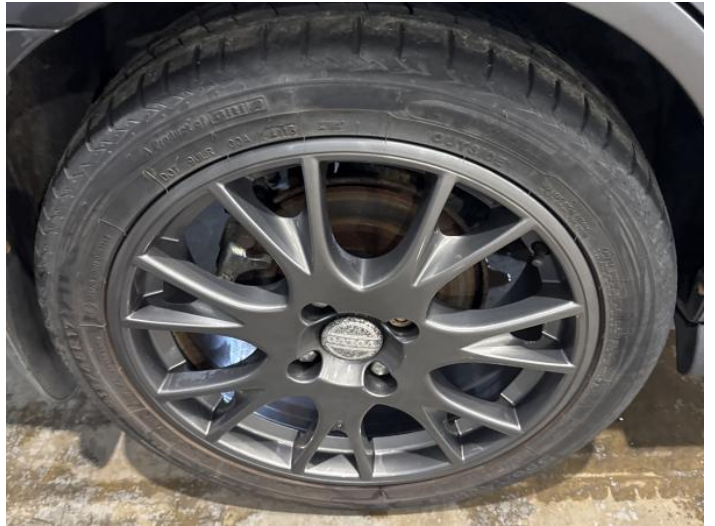
16: Wheel osr Scratched Up To 50mm
