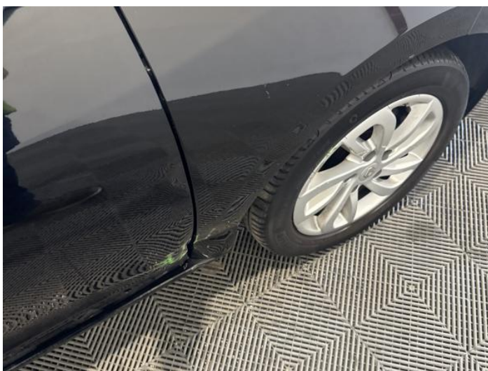
19: Wing osf Dented With Paint Damage
