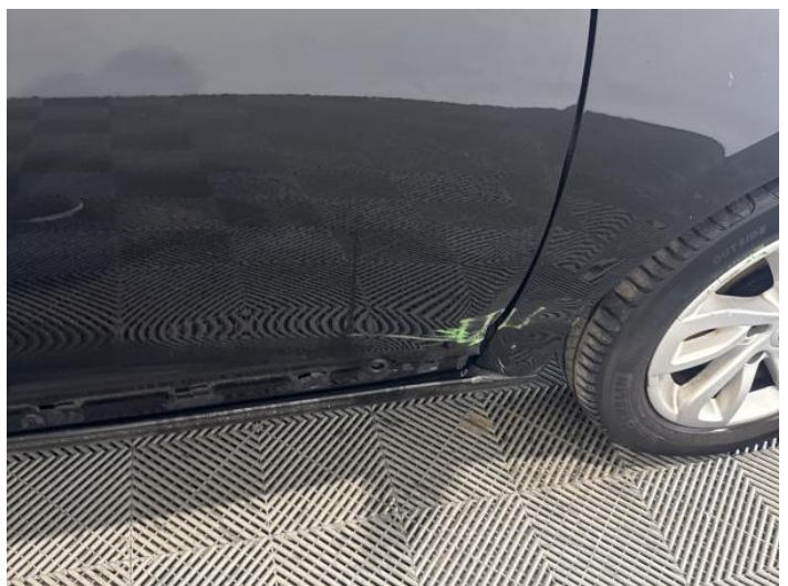
18: Door osf Dented With Paint Damage
