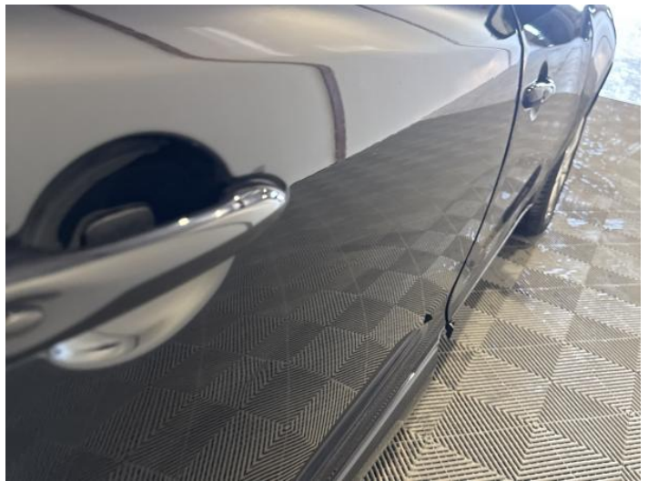
16: Door osr Dented Over 2 UpTo 10mm
