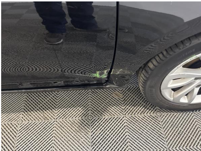
21: Sill os Dented With Paint Damage
