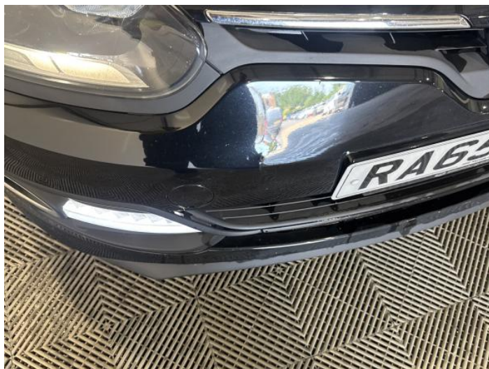
2: Bumper Front Dented With Paint Damage
