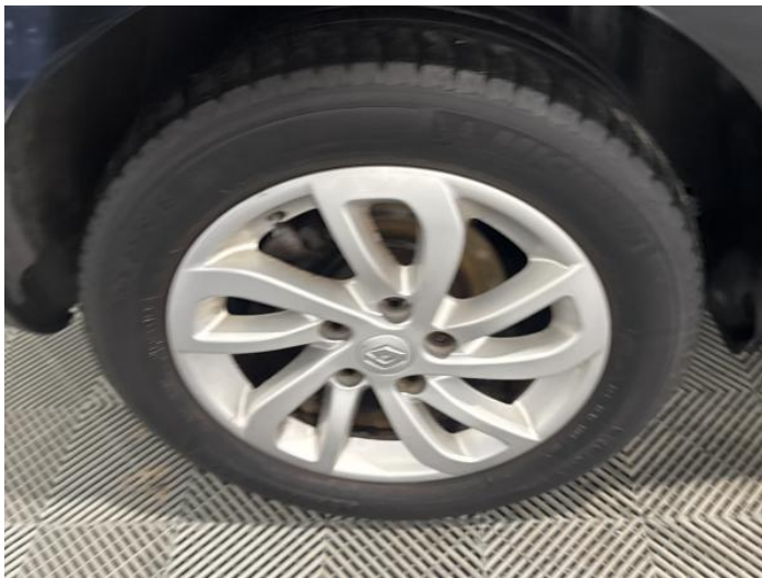
15: Wheel osr Scratched Up To 50mm
