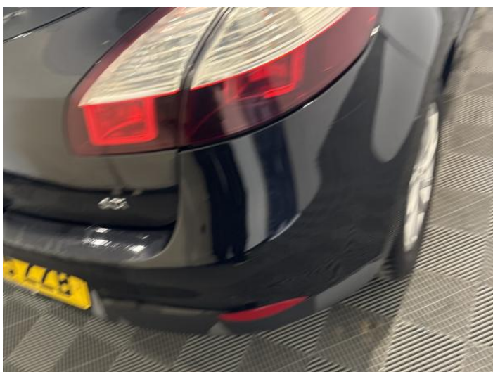
11: Bumper Rear Scratched 25 to 100mm Thru Paint
