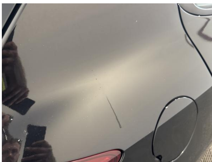
14: Qtr Panel osr Poor Previous Repair Poor Paint
