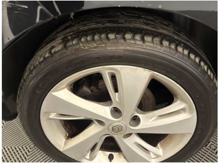
16: Wheel osr Scratched Over 50mm
