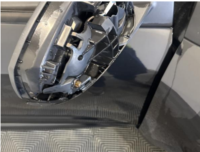
23: Door Mirror Assy osf Broken Replace
