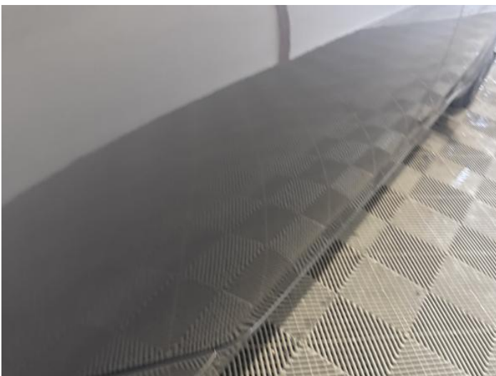
13: Door osr Dented Over 2 UpTo 10mm
