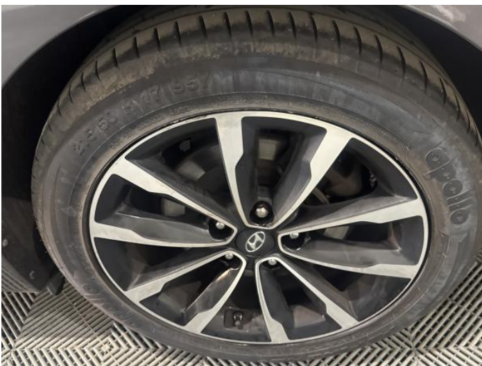
7: Wheel nsr Scratched Over 50mm
