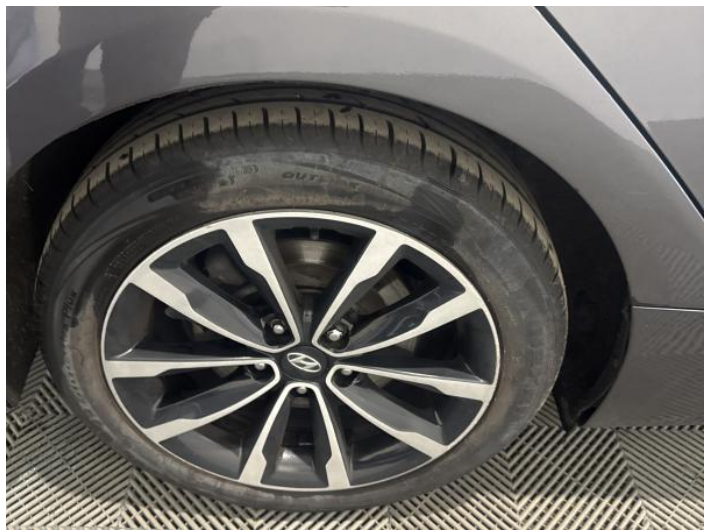
12: Wheel osr Scratched Up To 50mm
