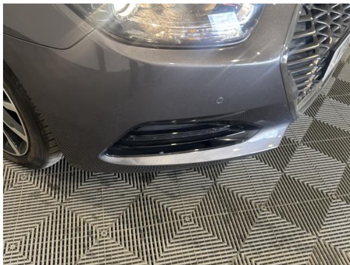
2: Bumper Front Scratched Over 100mm Thru Paint
