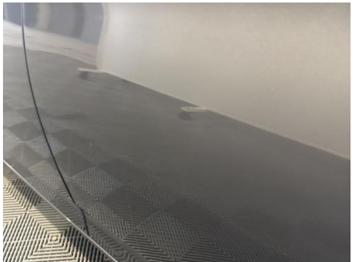
6: Door nsr Dented Between 10mm + 30mm
