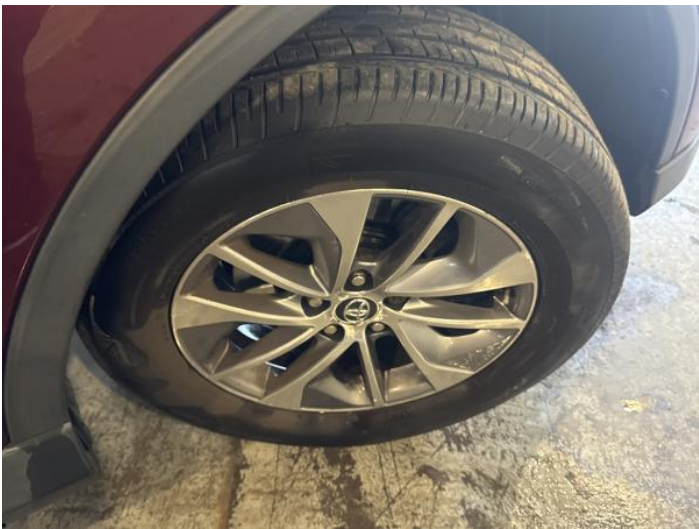
17: Wheel osf Scratched Over 50mm
