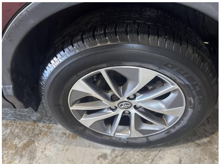
8: Wheel nsr Scratched Up To 50mm
