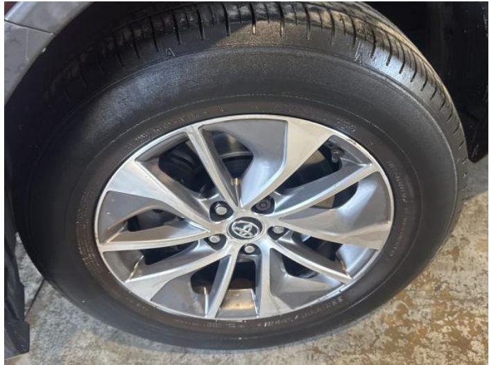
4: Wheel nsf Scratched Over 50mm
