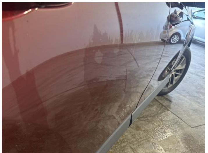
14: Door osr Dented Over 2 UpTo 10mm
