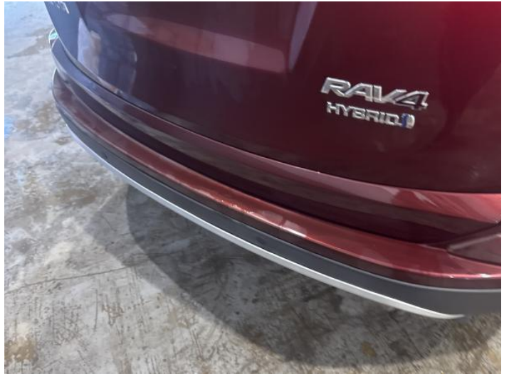
10: Bumper Rear Poor Previous Repair Paint Flake
