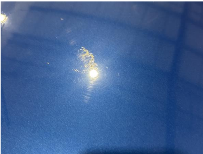
17: Roof Poor Previous Repair Paint Flake
