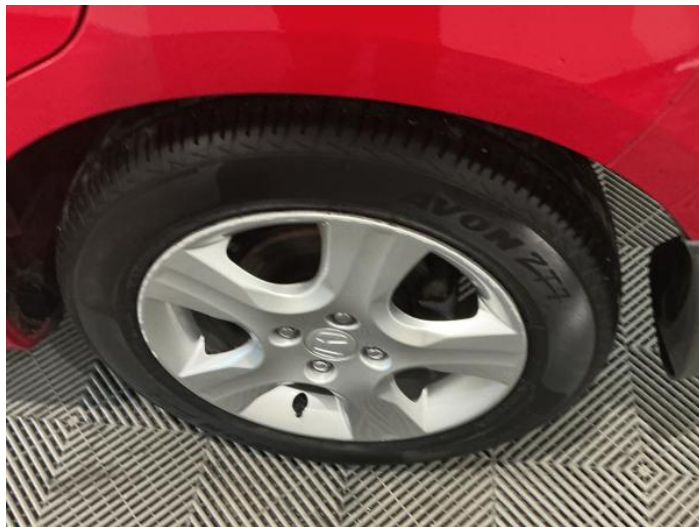
10: Wheel nsr Scratched Over 50mm
