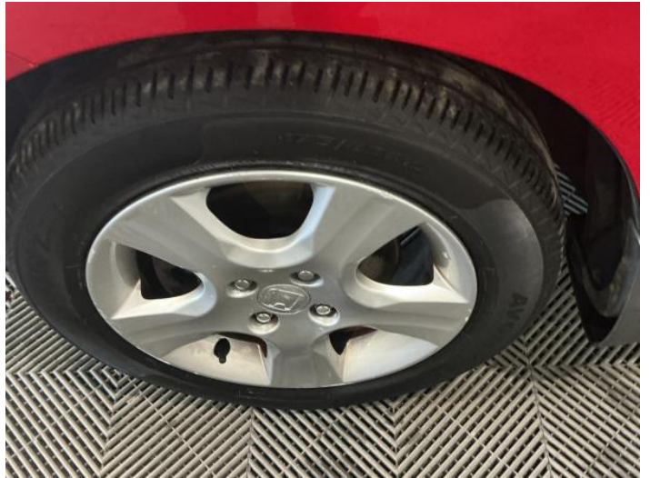
4: Wheel nsf Scratched Over 50mm
