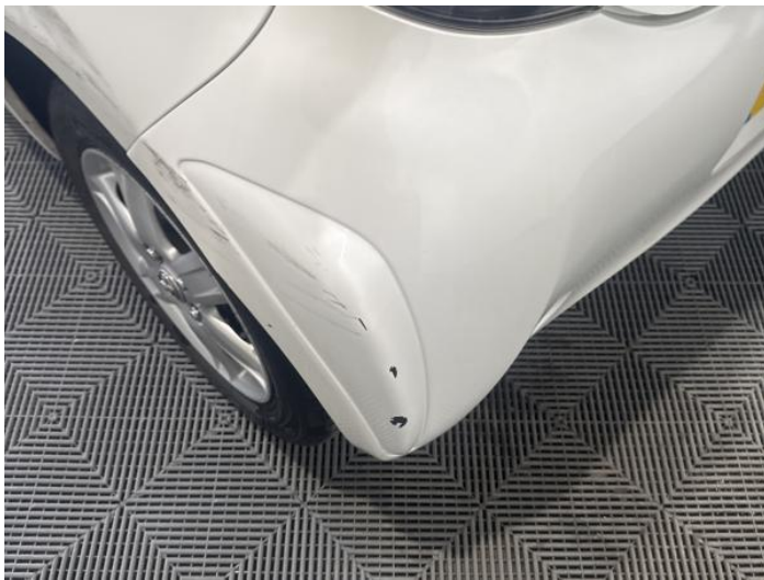
11: Bumper Rear Scratched Over 100mm Thru Paint
