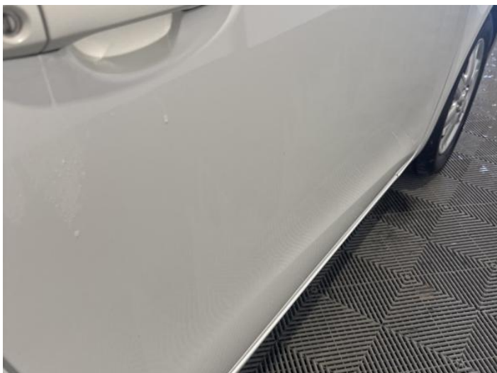
15: Door osf Dented Over 2 UpTo 10mm
