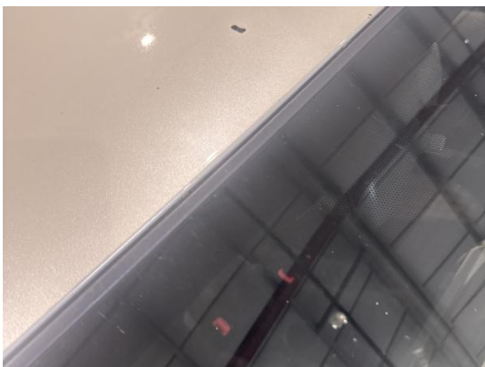
19: Roof Chipped Over 5mm
