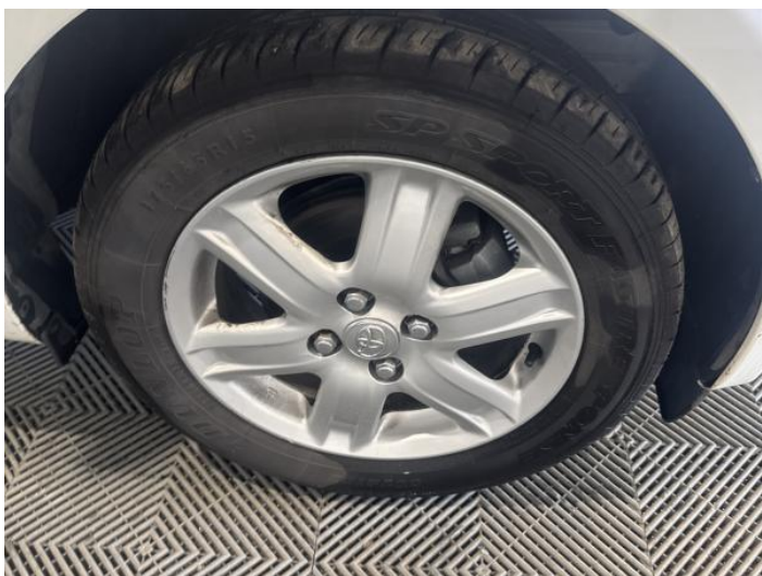
17: Wheel osf Scratched Up To 50mm
