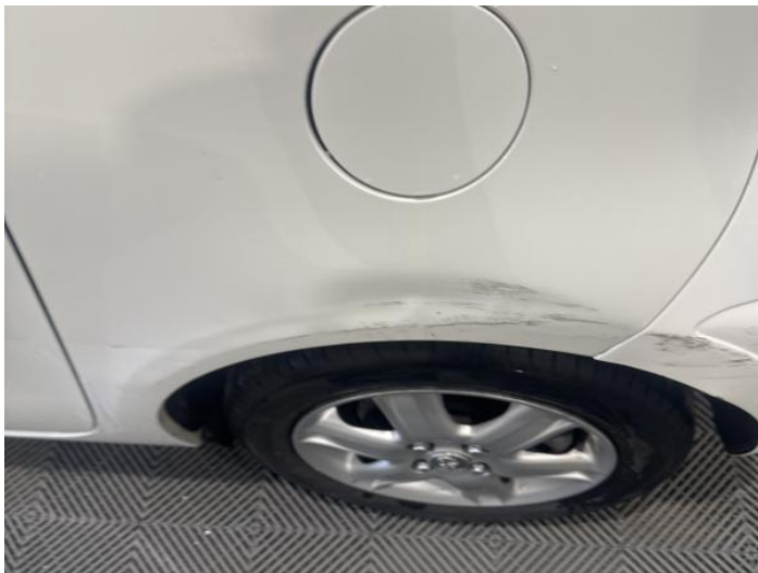
9: Qtr Panel nsr Dented With Paint Damage
