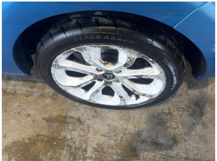
10: Wheel nsr Scratched Over 50mm
