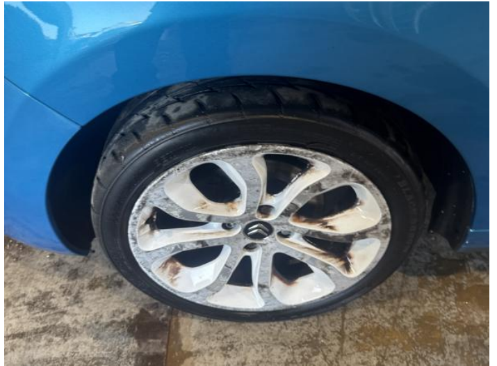
4: Wheel nsf Scratched Over 50mm
