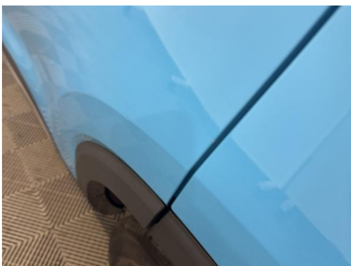
7: Door nsr Dented 2 Or Less UpTo 10mm
