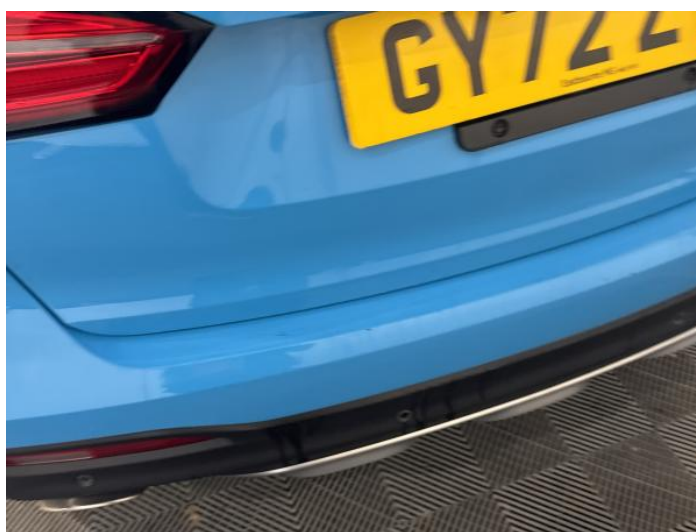
8: Bumper Rear Chipped Multiple Chips
