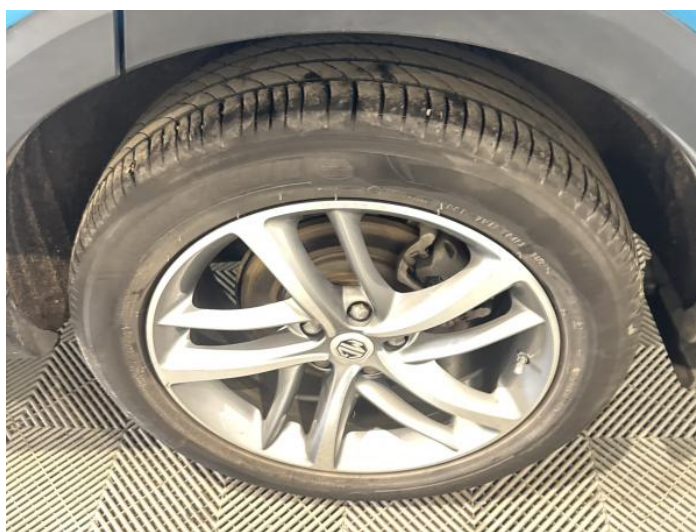
6: Wheel nsr Scratched Over 50mm
