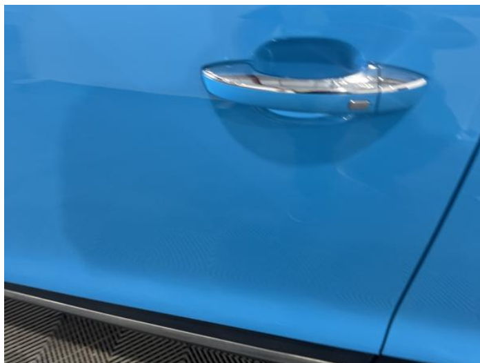
4: Door nsf Dented 2 Or Less UpTo 10mm
