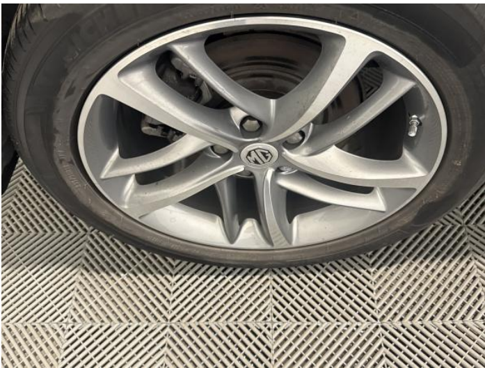
11: Wheel osr Scratched Up To 50mm
