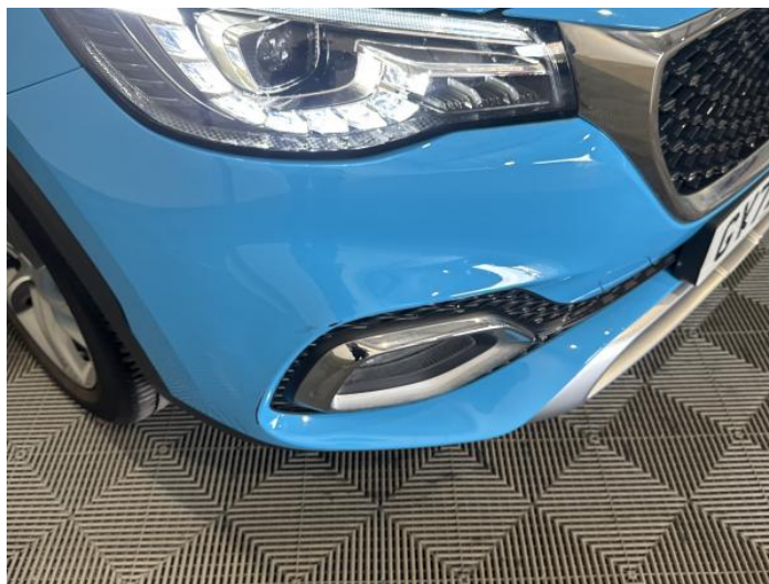
2: Bumper Front Scratched Over 100mm Thru Paint
