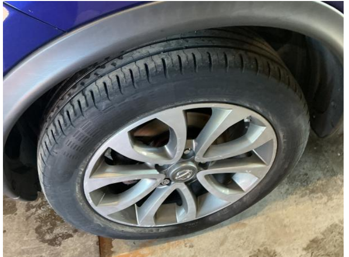
4: Wheel nsf Scratched Over 50mm
