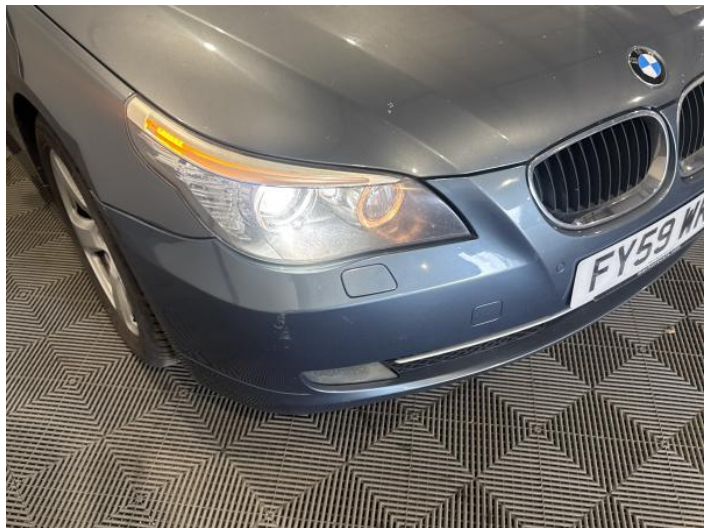
2: Bumper Front Scratched Over 100mm Thru Paint
