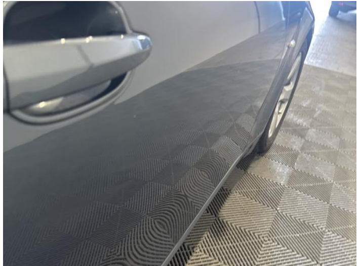
16: Door osf Dented Over 2 UpTo 10mm
