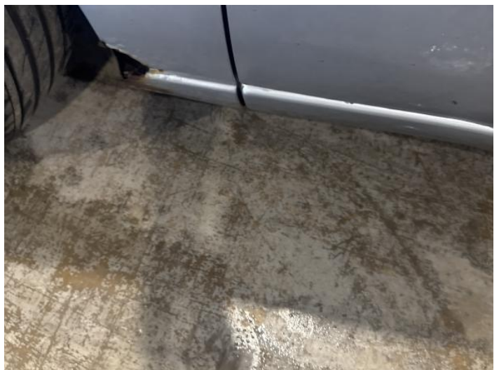
8: Sill ns Rusted Holed
