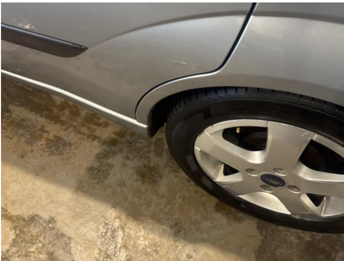
11: Qtr Panel nsr Rusted UpTo 5mm
