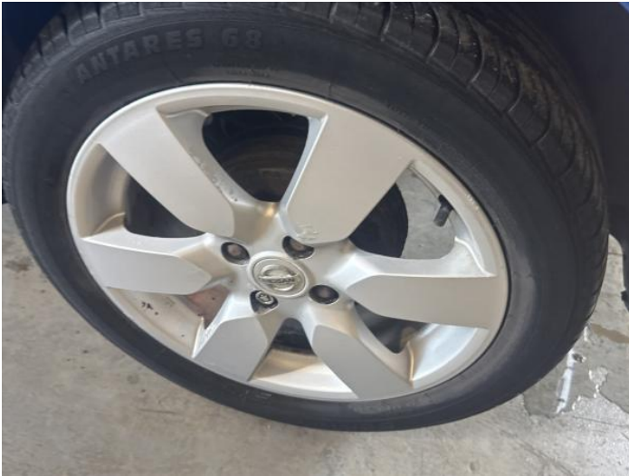
9: Wheel nsr Scratched Over 50mm
