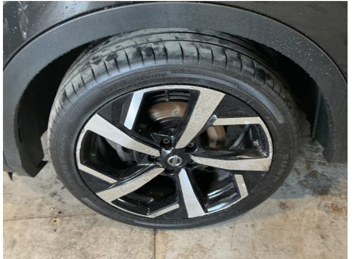
4: Wheel nsf Scratched Over 50mm
