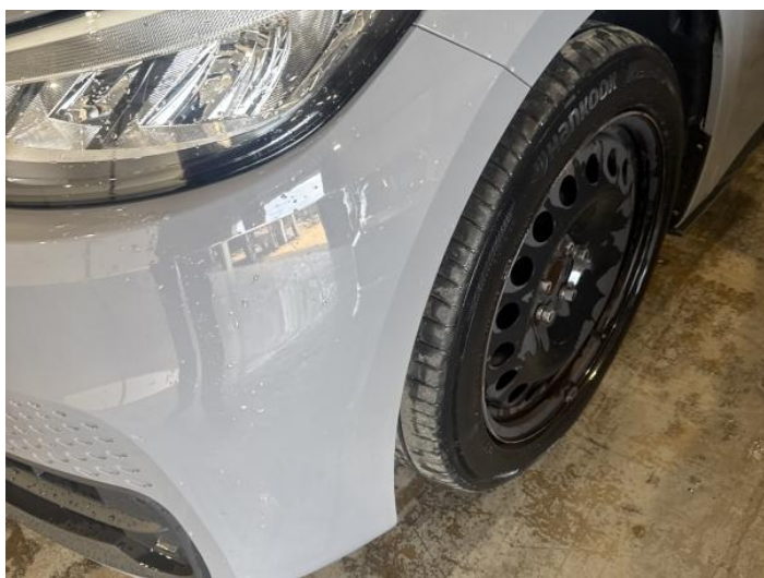
1: Bumper Front Scratched 25 to 100mm Thru Paint
