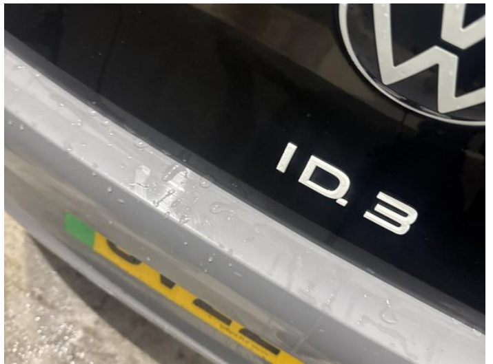
6: Bumper Rear Scratched 25 to 100mm Thru Paint
