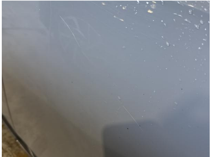
4: Door nsf Scratched Over 25mm Thru Paint
