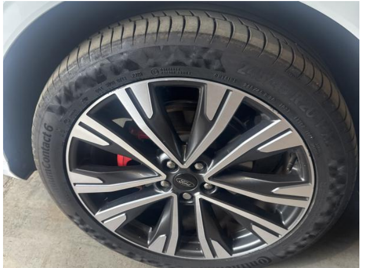
4: Wheel nsf Scratched Up To 50mm
