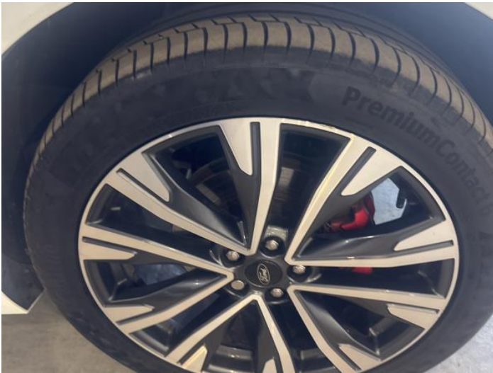
11: Wheel osf Scratched Up To 50mm
