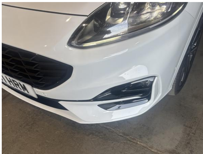
2: Bumper Front Chipped Multiple Chips
