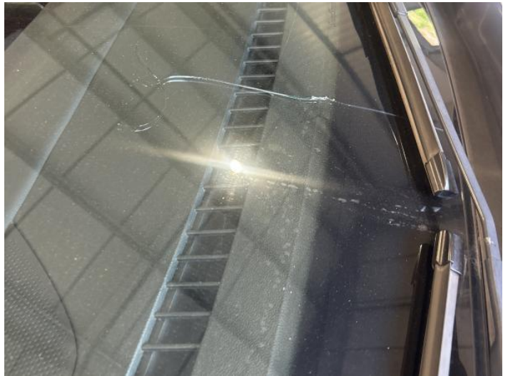
12: Screen Front Cracked Replace
