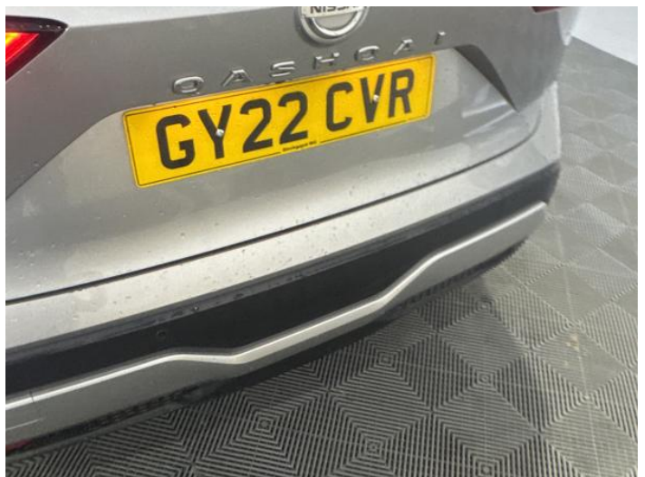
8: Bumper Rear Scratched 25 to 100mm Thru Paint
