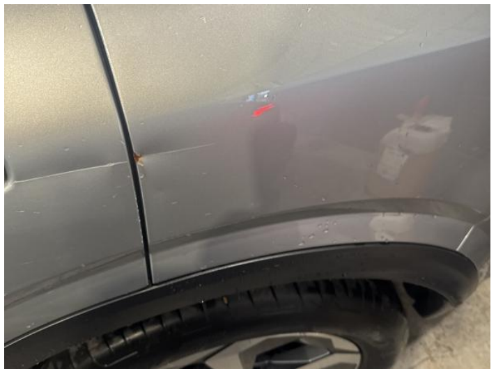
6: Qtr Panel nsr Dented With Paint Damage
