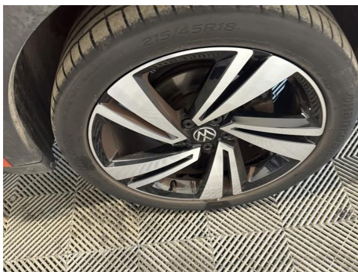
18: Wheel osf Scratched Up To 50mm
