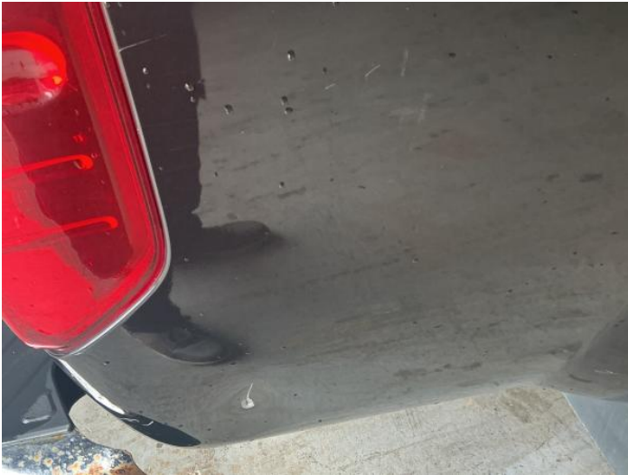
3: Qtr Panel osr Dented With Paint Damage
