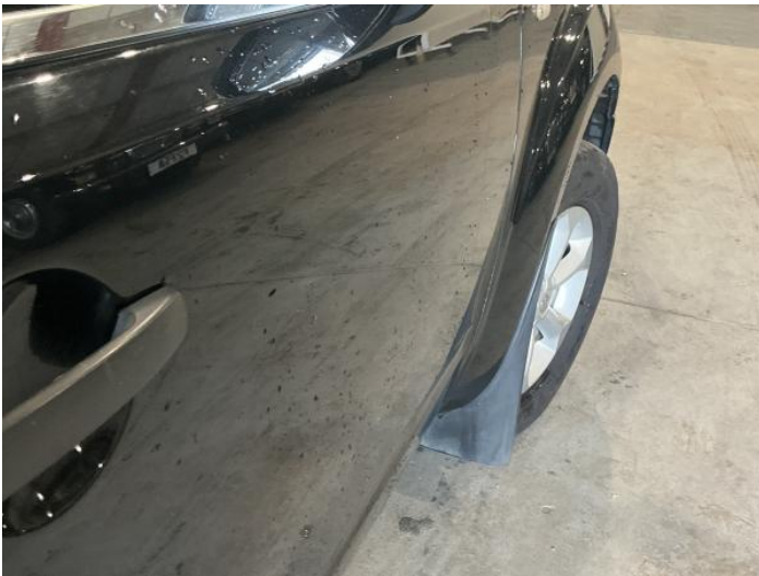
7: Door osf Dented Between 10mm + 30mm
