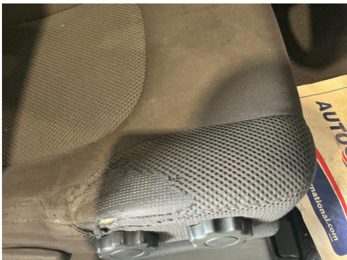
21: Seat Base Cover osf Torn Over 3mm
