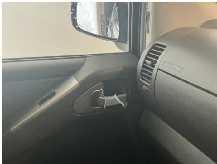
22: Handle Inner nsf Damaged Replace
