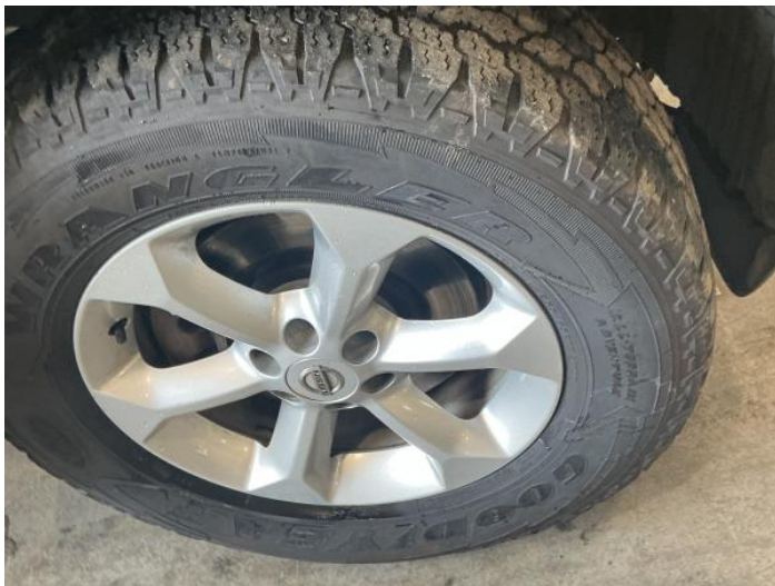
9: Wheel osf Scratched Over 50mm
