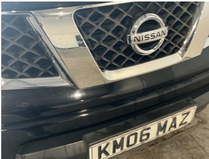
11: Bumper Front Poor Previous Repair Poor Paint
