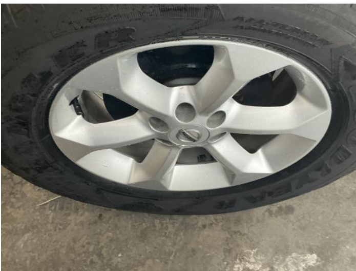
19: Wheel nsr Scratched Over 50mm
