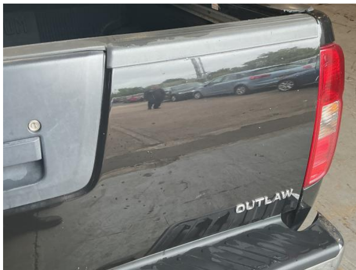
2: Boot Lid Dented With Paint Damage
