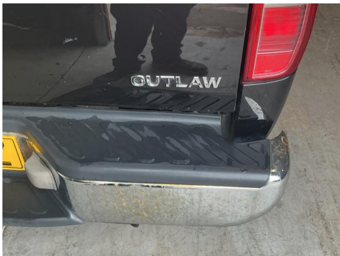
1: Bumper Rear Scratched Over 100mm Thru Paint
