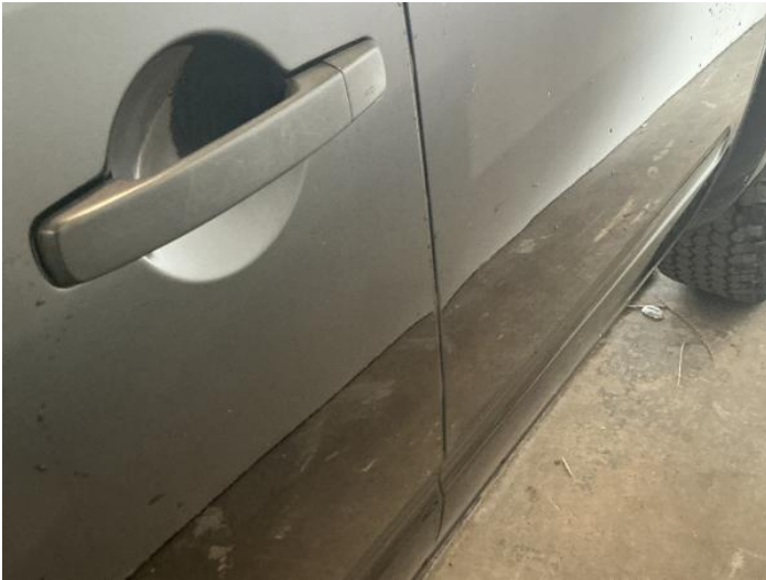
15: Door nsf Dented Between 10mm + 30mm
