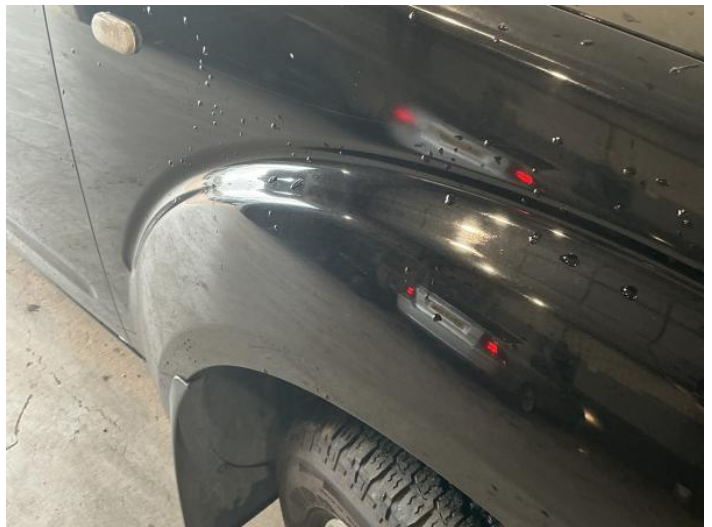
10: Wing osf Poor Previous Repair Poor Paint
