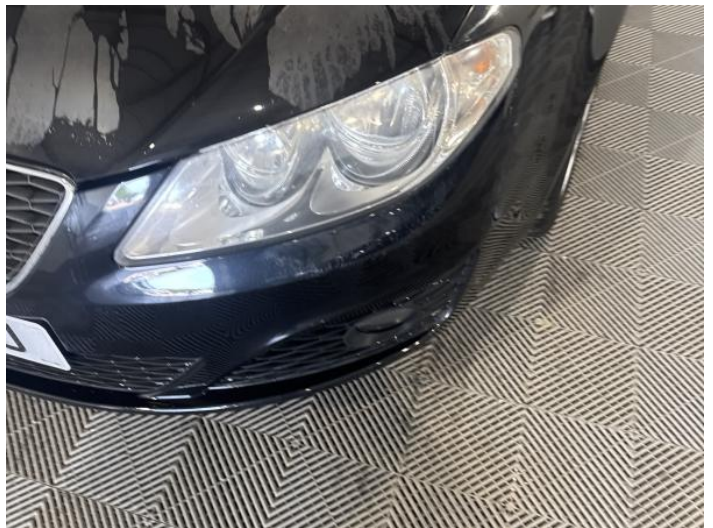
2: Bumper Front Scratched 25 to 100mm Thru Paint
