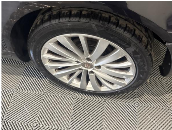
10: Wheel nsr Scratched Over 50mm
