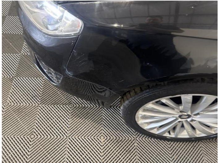
4: Wing nsf Scratched Over 25mm Thru Paint
