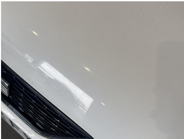
9: Bonnet Scratched Over 25mm Thru Paint
