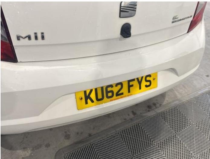
1: Bumper Rear Scratched 25 to 100mm Thru Paint
