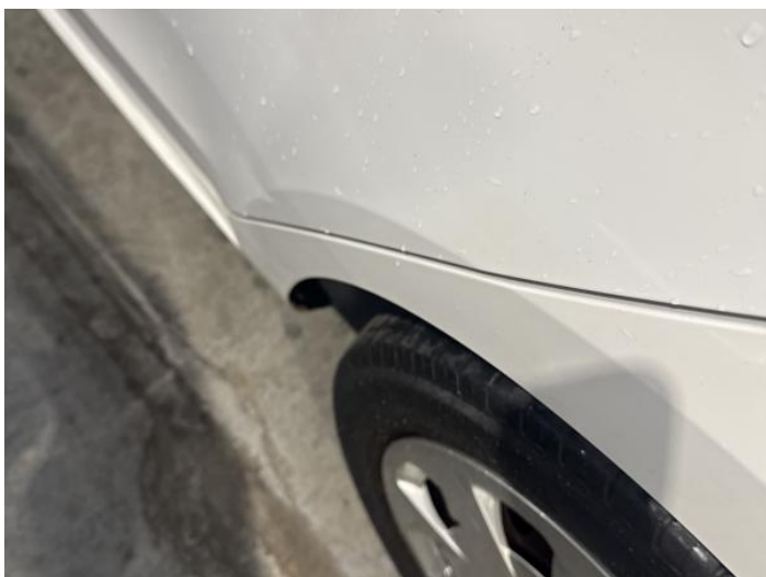
5: Door nsr Dented 2 Or Less UpTo 10mm
