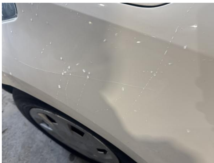
8: Wing nsf Scratched Over 25mm Thru Paint
