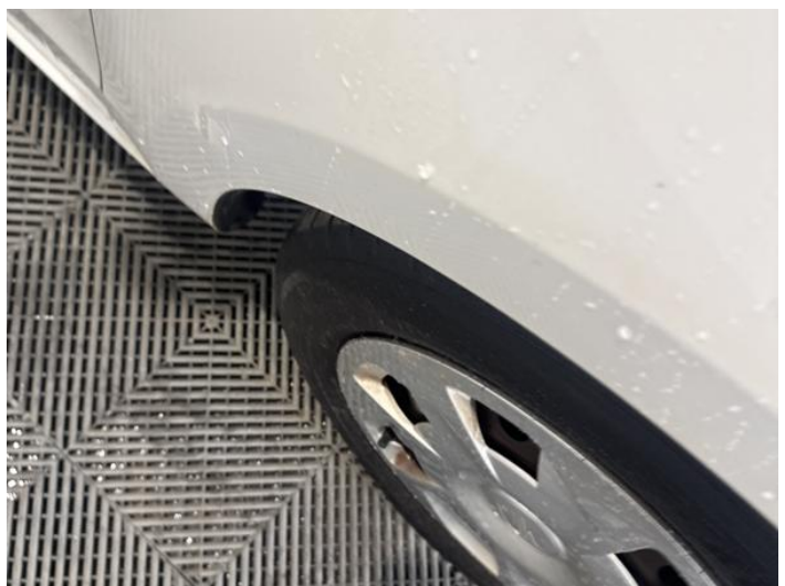
12: Wing osf Rusted UpTo 5mm
