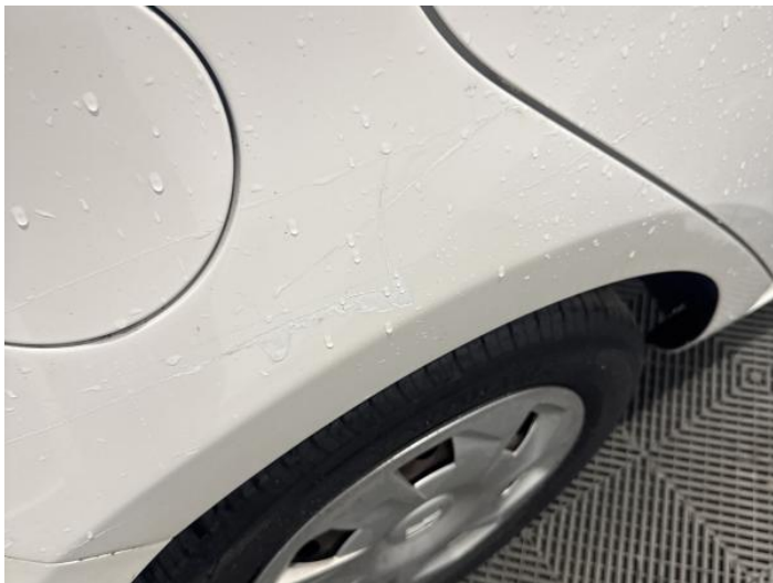
15: Qtr Panel osr Poor Previous Repair Paint Flake
