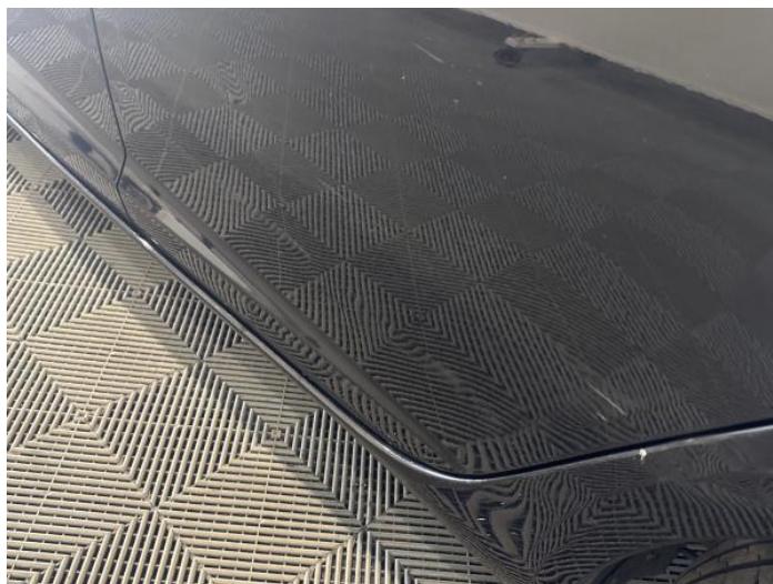
10: Door nsr Dented With Paint Damage
