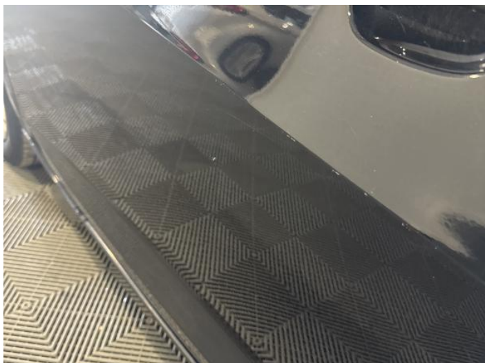
9: Door nsf Dented With Paint Damage
