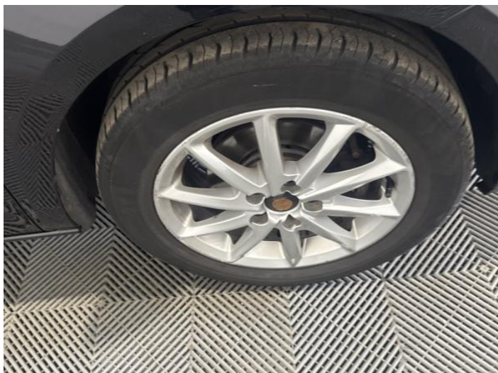
21: Wheel of Scratched Over 50mm
