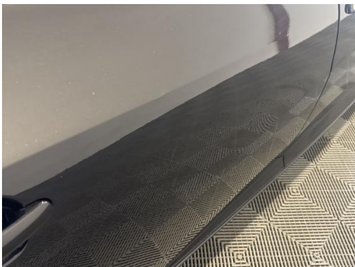
17: Door osr Dented With Paint Damage
