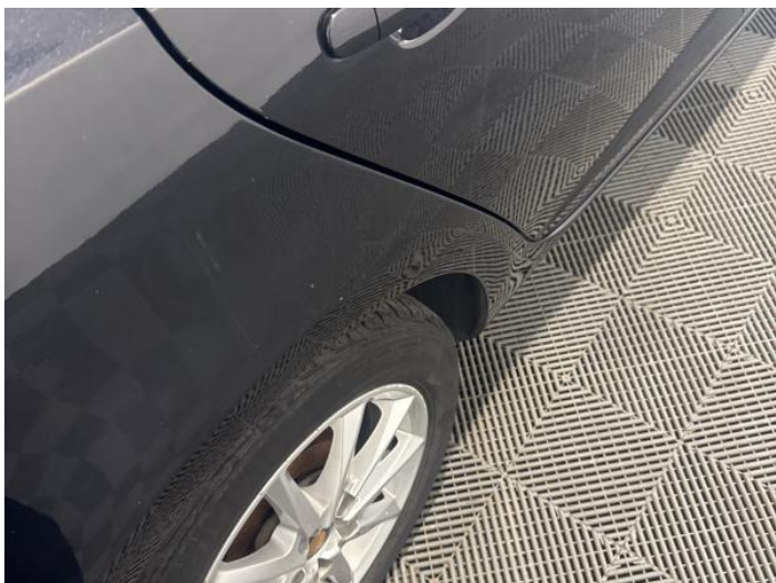
15: Qtr Panel osr Dented Over 30mm
