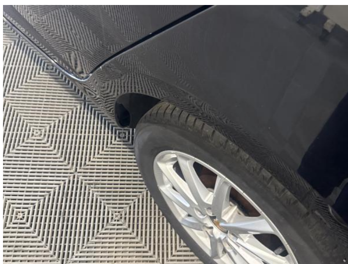
12: Qtr Panel nsr Dented With Paint Damage
