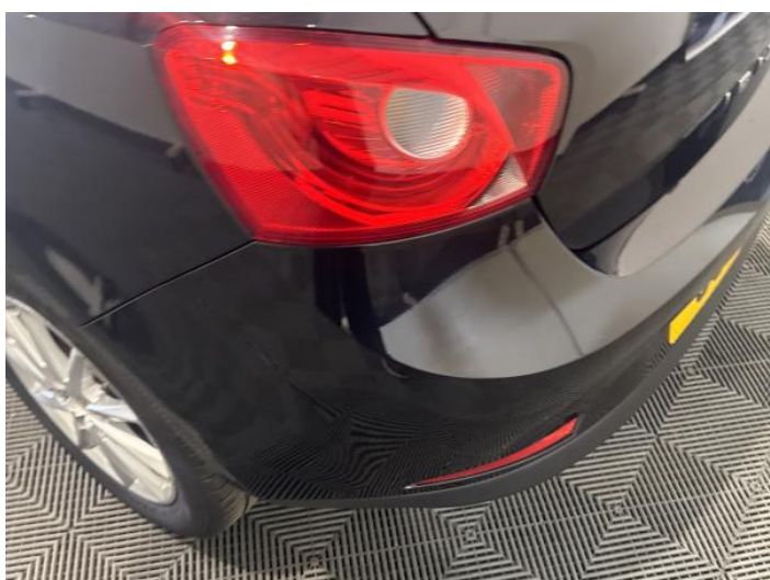
13: Bumper Rear Scratched Over 100mm Thru Paint
