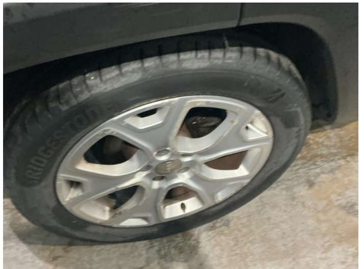
6: Wheel osr Scratched Over 50mm
