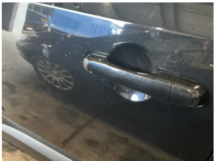
18: Door nsf Dented With Paint Damage
