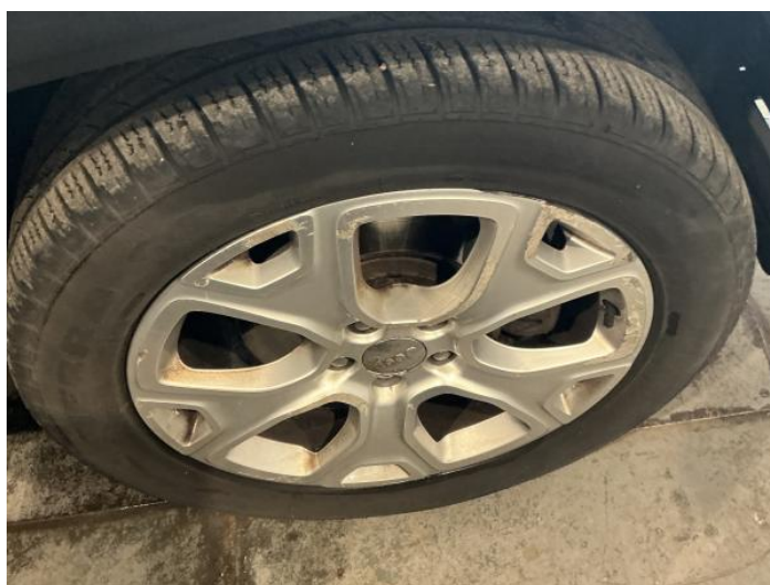
12: Wheel osf Scratched Over 50mm
