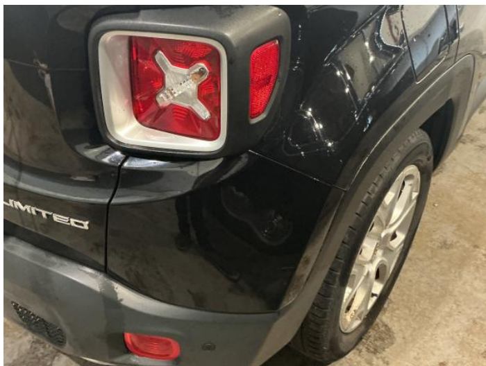
1: Bumper Rear Scratched 25 to 100mm Thru Paint
