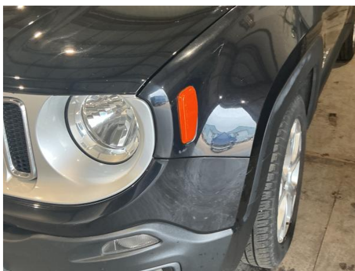
14: Bumper Front Scratched Over 100mm Thru Paint
