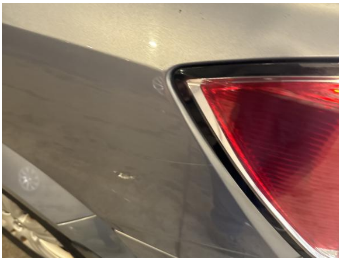
17: Qtr Panel nsr Scratched Over 25mm Thru Paint
