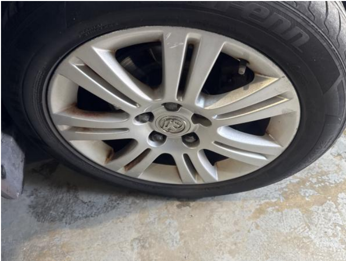
9: Wheel osf Scratched Over 50mm
