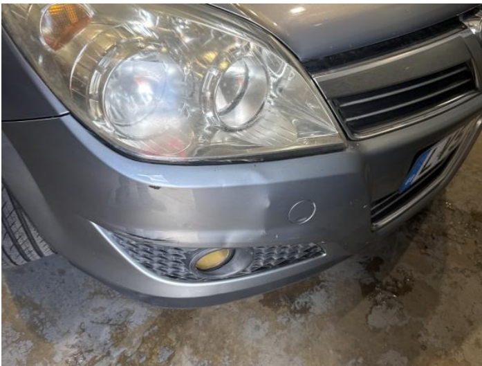
11: Bumper Front Dented With Paint Damage
