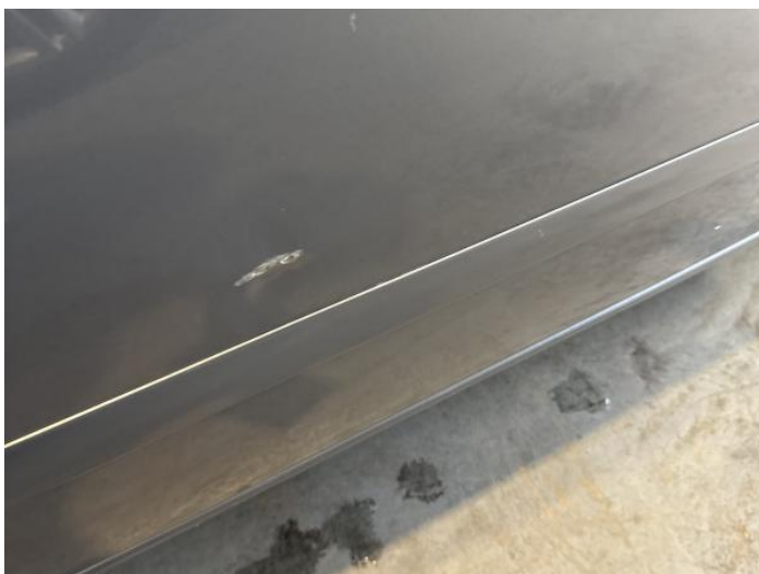
6: Door osf Dented With Paint Damage
