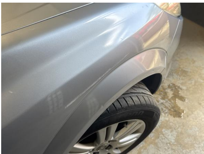
8: Wing osf Poor Previous Repair Poor Paint
