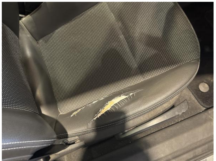
18: Seat Base Cover osf Torn Over 3mm
