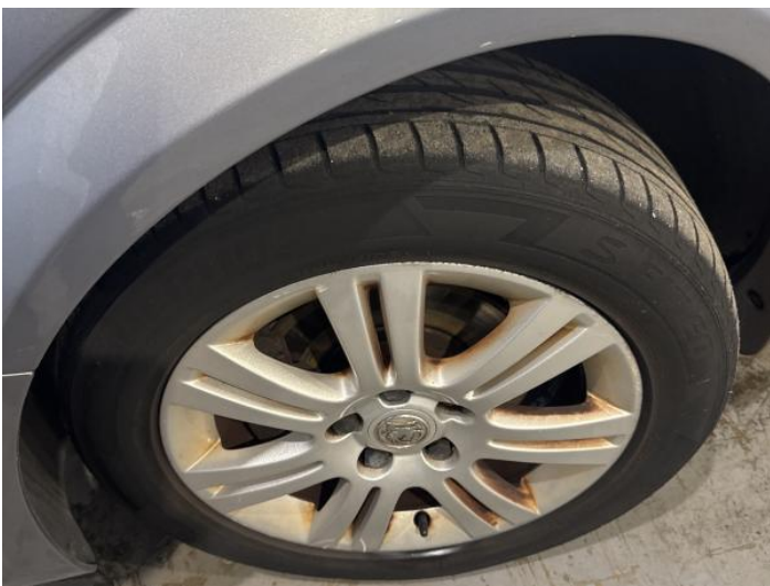
13: Wheel nsf Scratched Over 50mm
