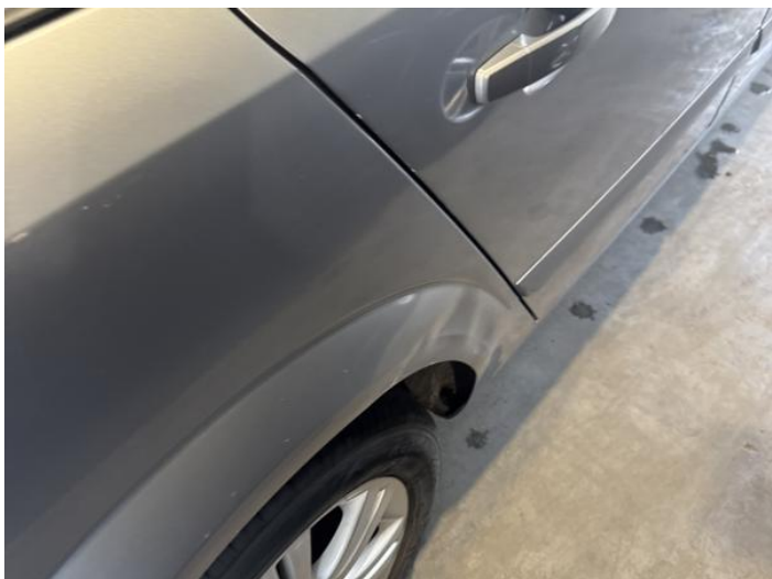
3: Qtr Panel osr Dented Over 30mm
