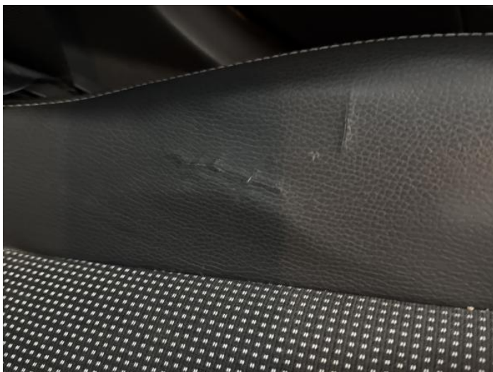
19: Seat Base Cover nsf Torn UpTo 3mm
