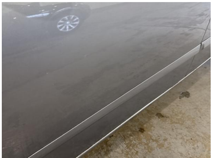
14: Door nsf Dented 2 Or Less UpTo 10mm
