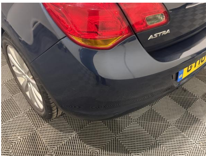
13: Bumper Rear Dented With Paint Damage
