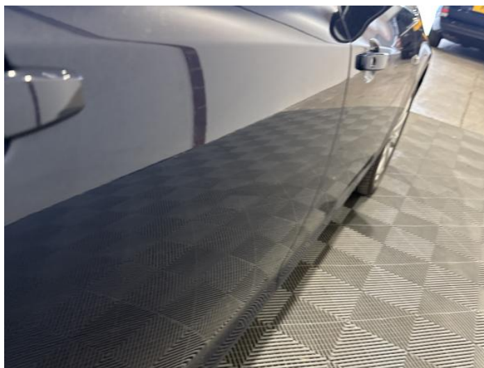
18: Door osr Dented Over 2 UpTo 10mm
