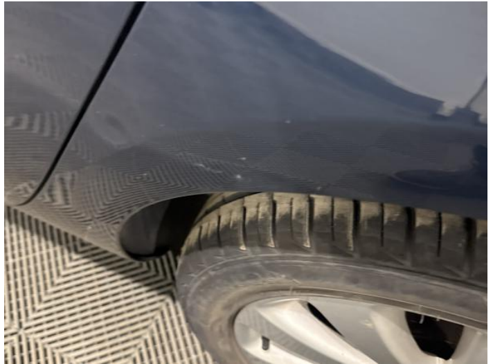
10: Qtr Panel nsr Dented Over 2 UpTo 10mm
