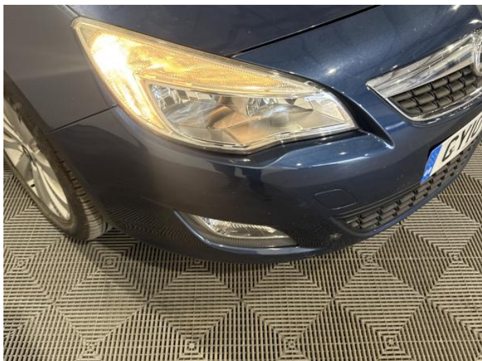
3: Bumper Front Scratched Over 100mm Thru Paint
