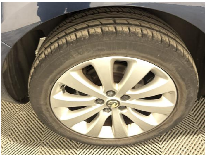
17: Wheel osr Scratched Over 50mm
