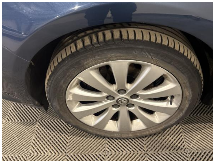
4: Wheel nsf Scratched Over 50mm
