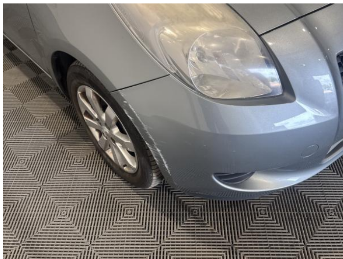
2: Bumper Front Scratched Over 100mm Thru Paint
