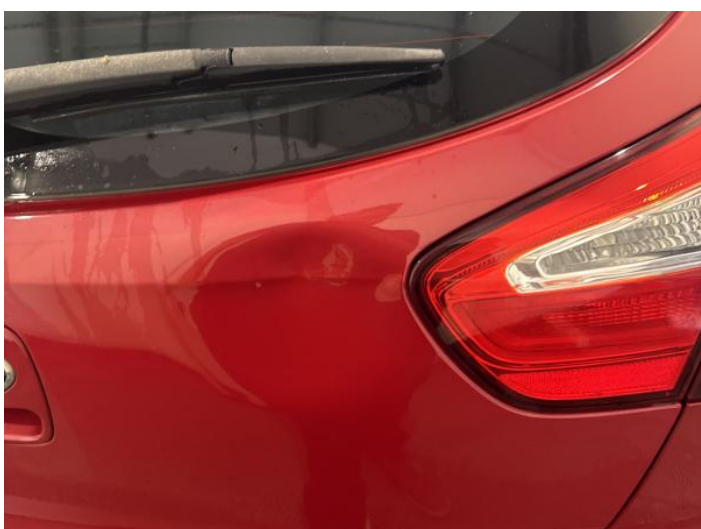
13: Boot Lid Dented Over 30mm
