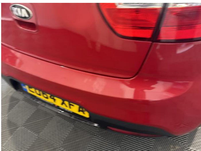
11: Bumper Rear Scratched 25 to 100mm Thru Paint
