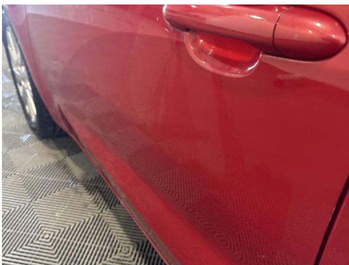
7: Door nsf Dented Over 30mm
