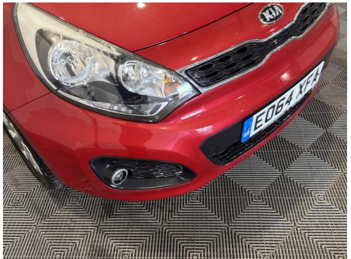
2: Bumper Front Chipped Multiple Chips
