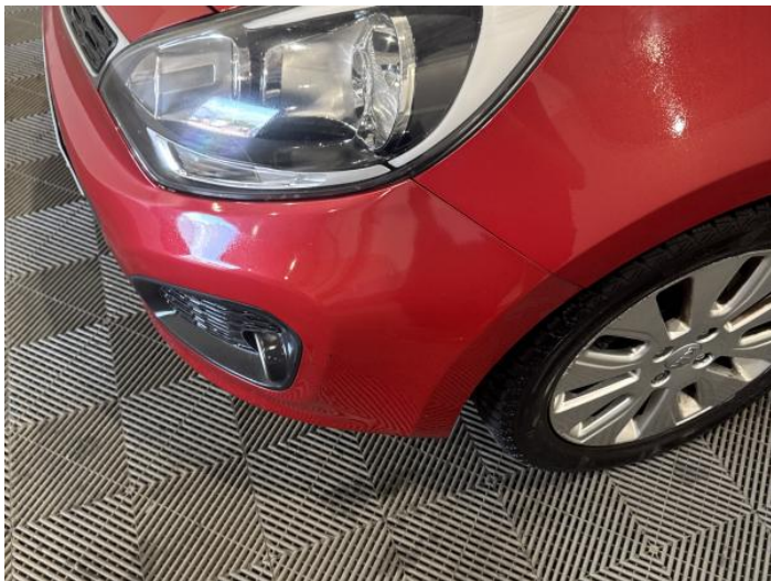
3: Bumper Front Scratched 25 to 100mm Thru Paint
