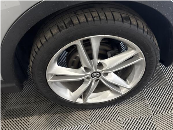
15: Wheel osf Scratched Over 50mm
