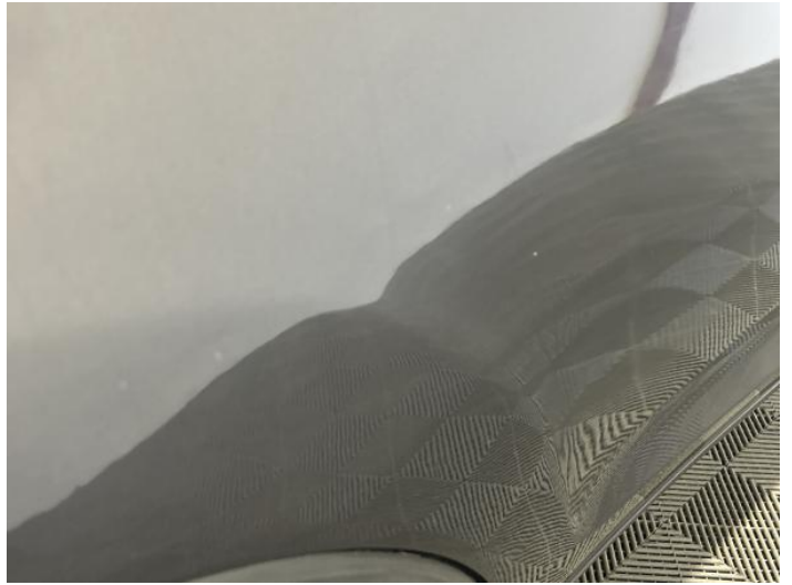
4: Door osr Poor Previous Repair Poor Paint
