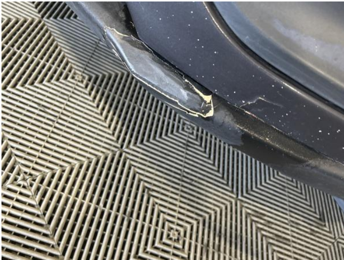
12: Bumper Front Moulding Broken Replace
