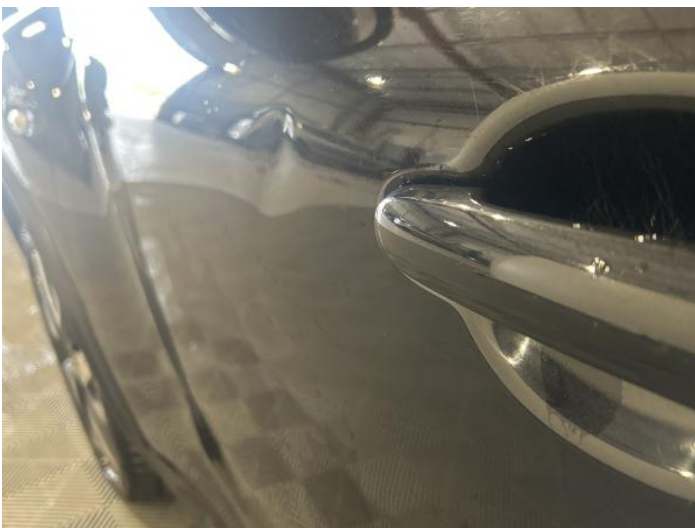
13: Door nsf Dented Over 30mm
