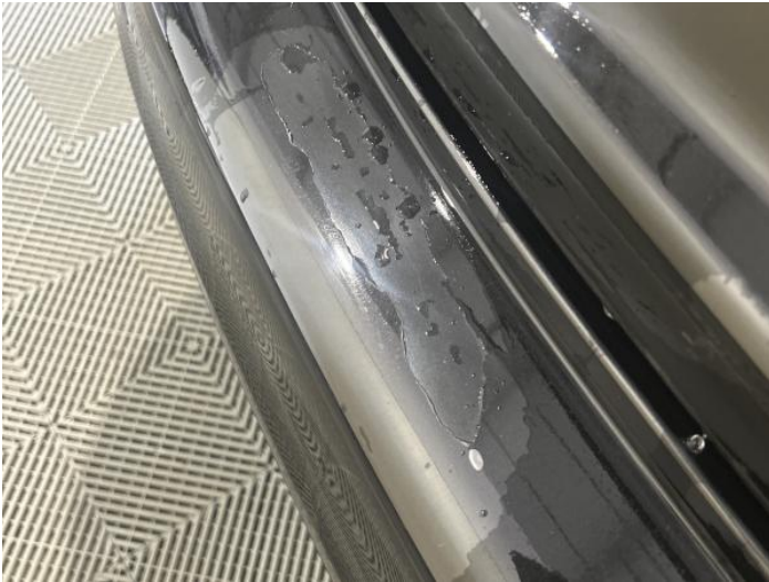
9: Bumper Rear Poor Previous Repair Paint Flake
