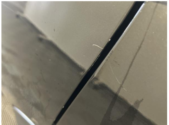
12: Door nsr Scratched UpTo 25mm Thru Paint
