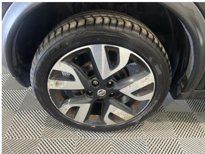
4: Wheel nsf Corroded Light
