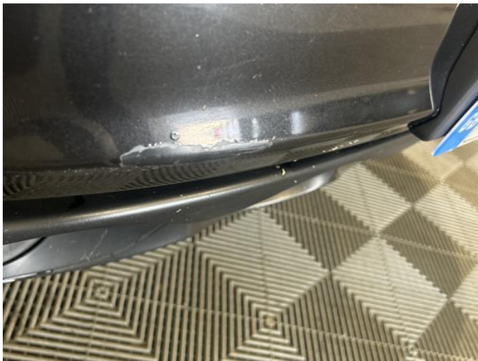
15: Bumper Front Poor Previous Repair Paint Flake
